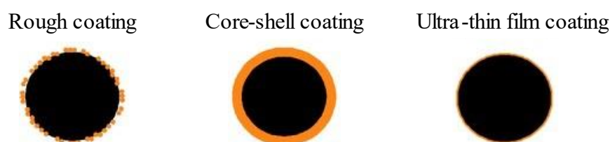
Figure 2.16: Schematic depicting three different coating characteristics: rough, core-shell and ultra-thin film coating. Adapted from [102]
