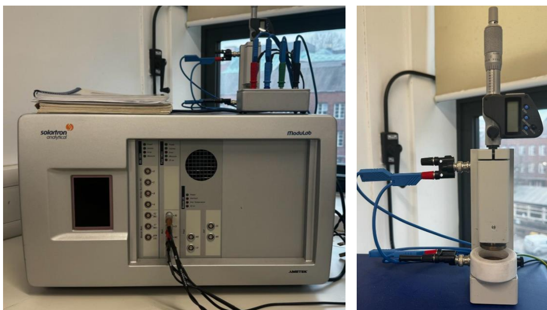
Figure 3.8: Electrochemical impedance spectroscopy set up showing the ModuLab XM ECS (left) and dedicated liquid sample holder (right).
