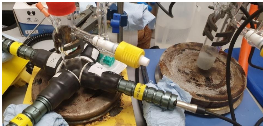
Figure 6.3: A photo shows two experimental setups of photochemical Giese reaction using one torch and four torches.
