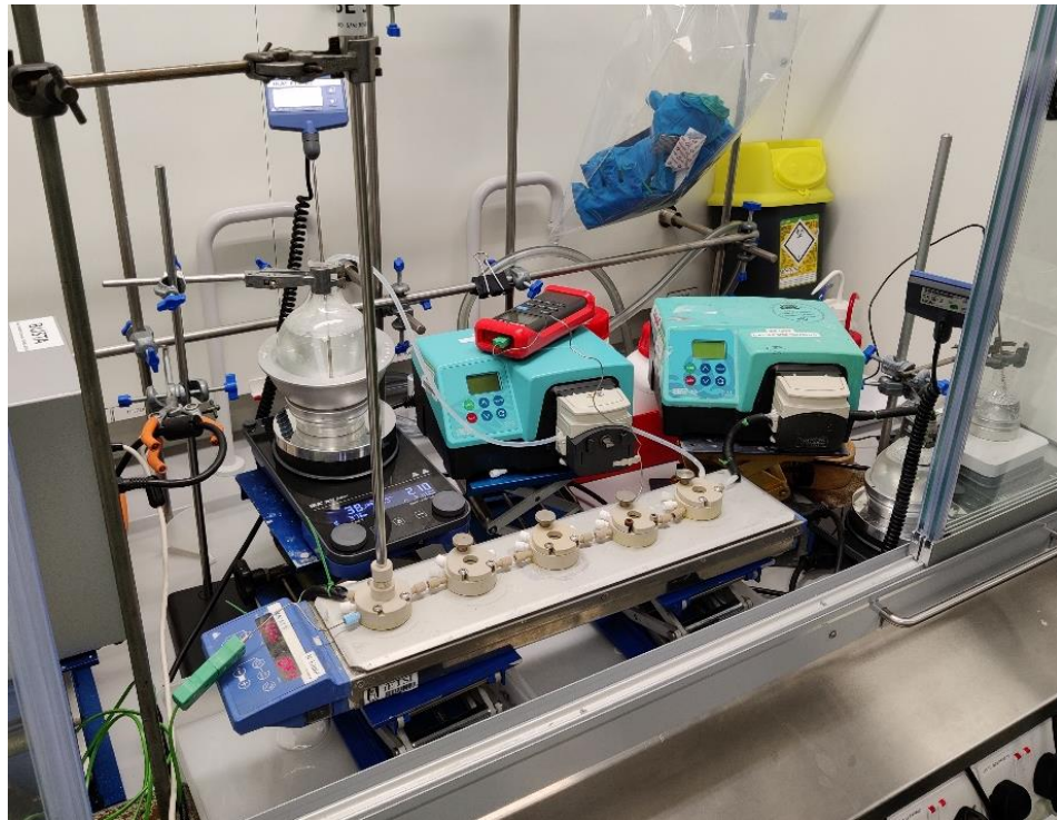
Figure 81 – Photograph of the apparatus used for the continuous seeded crystallisation experiments, showing the fReactor, pumps, and storage vessels.
