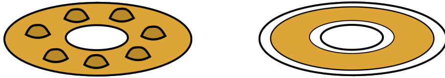
Figure 6.38: Grease presence when applied (left) vs presence during a test (right)
