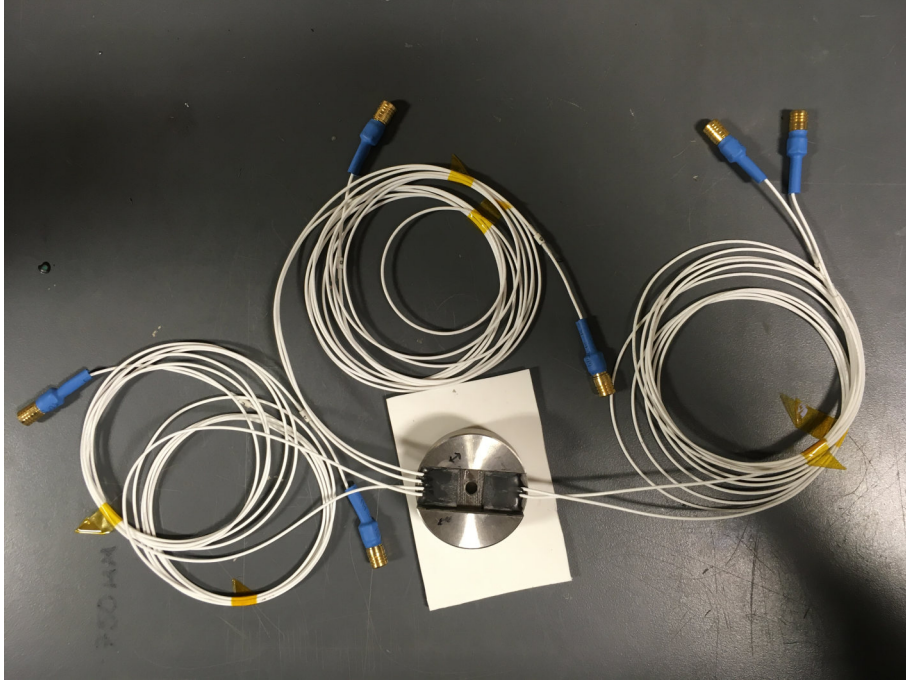
Figure 5.24: Upper specimen complete with SMB connectors and black Robnor potting compound
