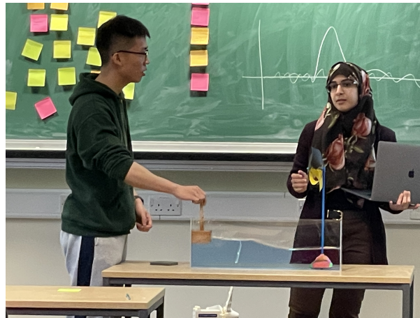
Figure 8.5: Wajiha and Yang while demonstrating the standing waves experimentally. The standing waves were produced in the scaled wavetank to demonstrate that the results obtained by the theoretical model (exact solution) and numerical solution were aligned with the experiments.
