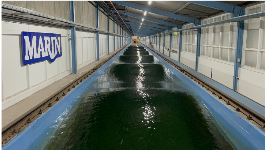
(a) Regular water waves generated in a rectangular wavetank at MARIN. Photo courtesy of MARIN.
