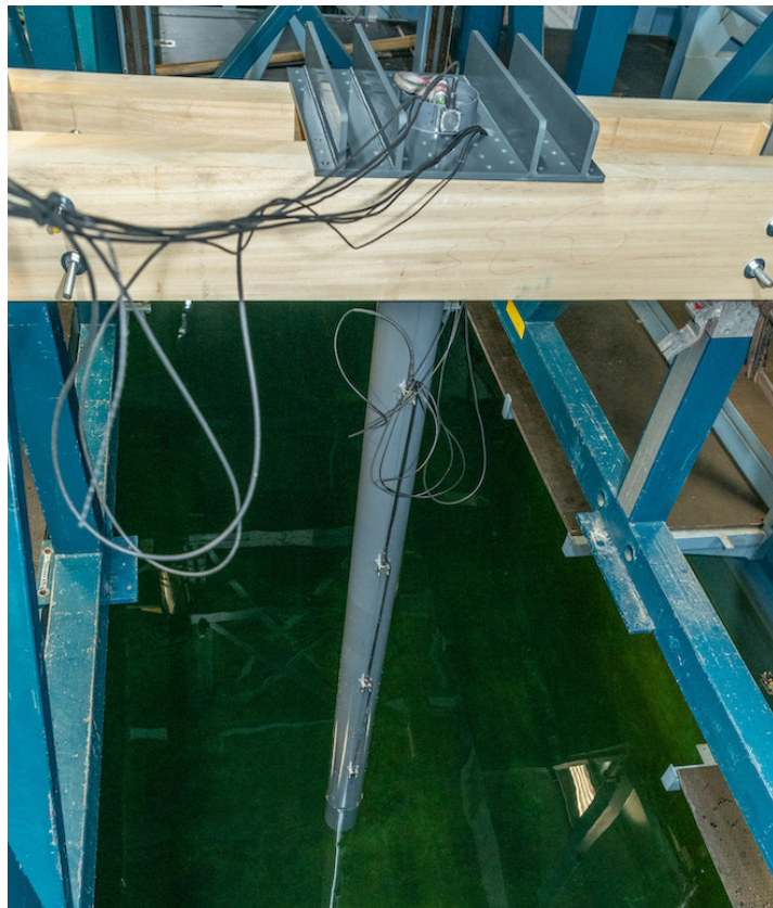
Figure 4.5: Baseplate, wooden support, beam, accelerometers and cables of the beam. See text for details.
