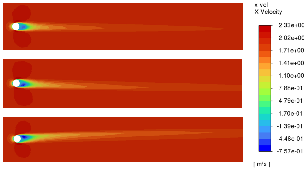
Figure 3.12 Flow velocity in x-axis of the mesh sensitivity study. From top to bottom: P1, P2, P3.
