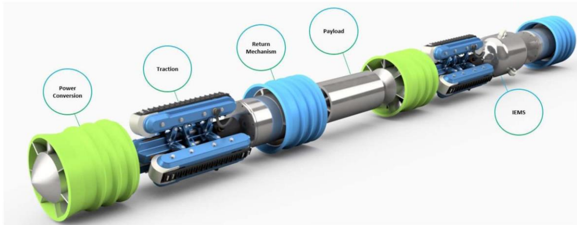
Figure 2.12 Illustration of a modular hybrid robot that combines tracked and PIG type (From [41]).
