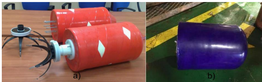
Figure 2.2 Examples of low cost PIGs. a) Low-cost foam PIGs with a six arms calliper (From [6]). b) Cleaning PIG (From [15]).
