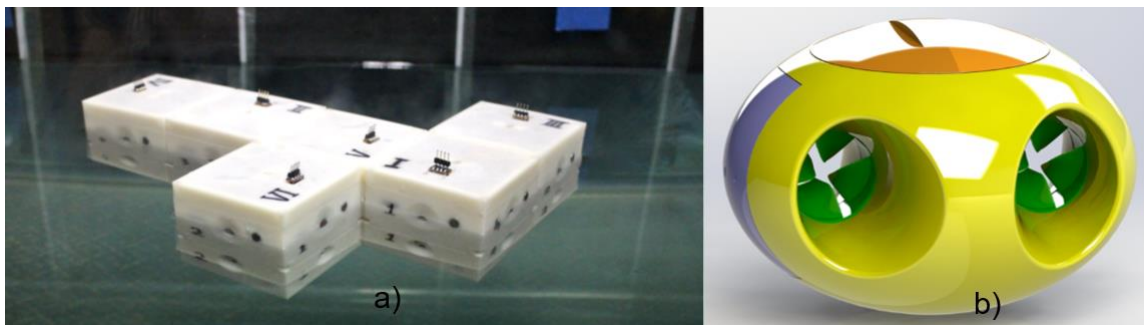
Figure 2.14 Propeller type robots. a) Prototype of a 2D modular robot with 6 modules (from [43]). b) Propeller type robot with two thrusters (from [44]).
