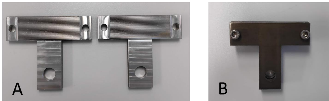
Figure 2.16 - The clamp used to grip the dehydrated surface of the porcine subscapularis tissue. (A) Ridged inner surface of the clamp. (B) Clamp assembled.
