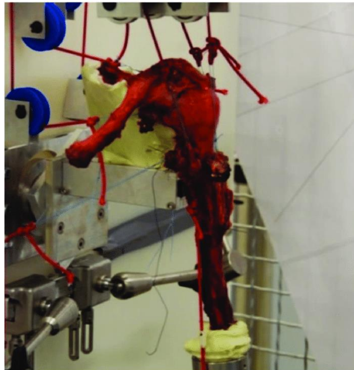
Figure 1.10 – The Aachen shoulder simulator. Six pneumatic muscles provide active motion of a cadaveric shoulder (Verjans et al., 2016). Image reproduced under the creative commons attribution license.
