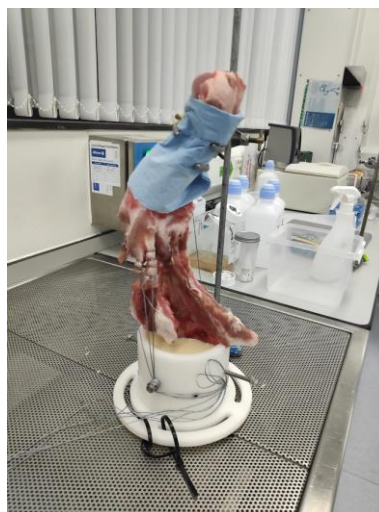
Figure 4.20 - Clamp was used in order to allow for the cementing of the scapula into the simulator fixture.
