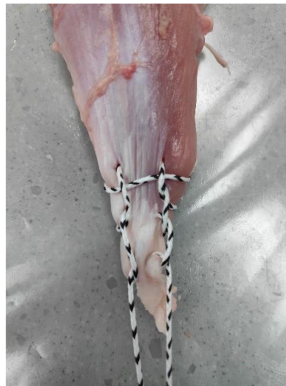
Figure 2.5 - The Krackow whip stitch on a porcine tendon of the short head of the biceps using the Dorisea extreme braid fishing line.
