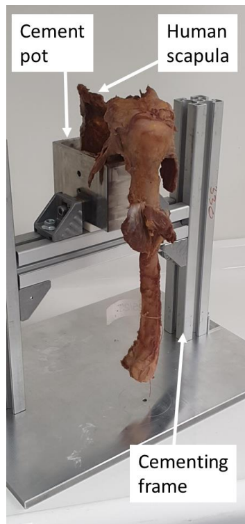
Figure 5.7 - The custom made cementing fixture during the cementing process.
