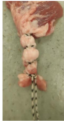
Figure 2.6 - The modified finger trap stitch on a porcine tendon of the long head of the biceps using Dorisea extreme braid fishing line.
