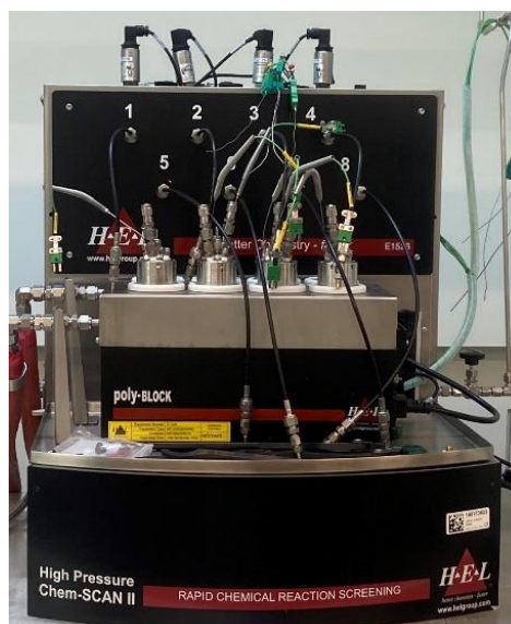
Figure 60. Image of the H.E.L. HP ChemSCAN used in the catalyst screen for the reduction of osimertinib nitrodiamine.
