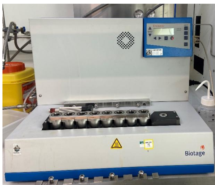
Figure 61. The Biotage Endeavor catalyst screening platform used in the kinetic experiments.
