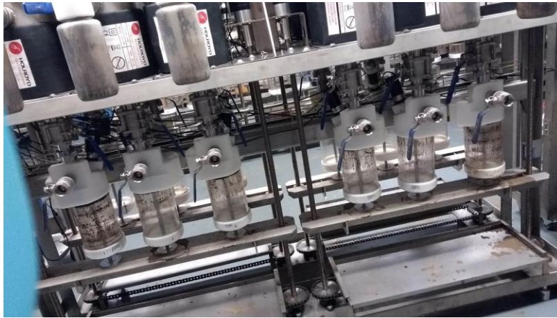
Figure 3.2 - The O-rings within the plungers of the feed syringes were not suitable for use with high particulate feedstocks.
