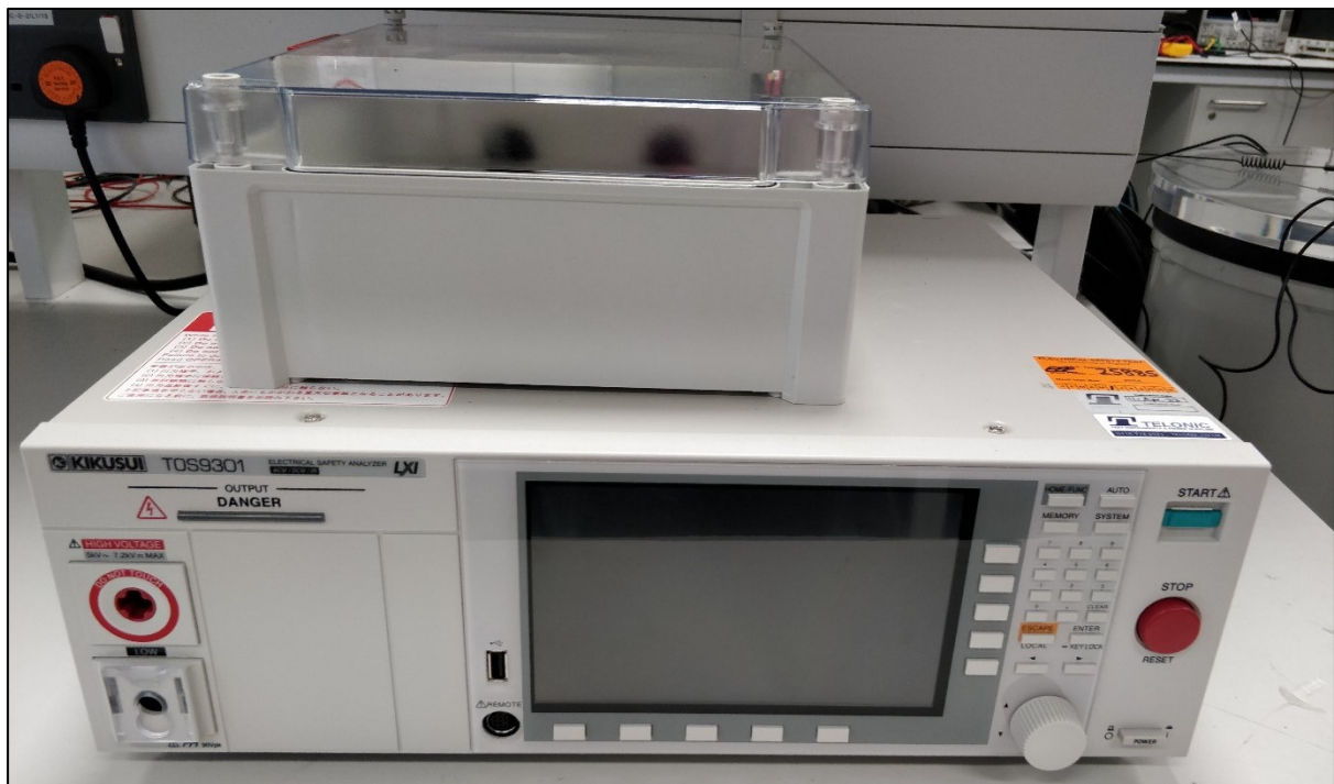
Fig. 5.17 Photograph of Kikusui TOS9301 electrical safety tester used for the generation of PD under 50 Hz AC stimulus.
