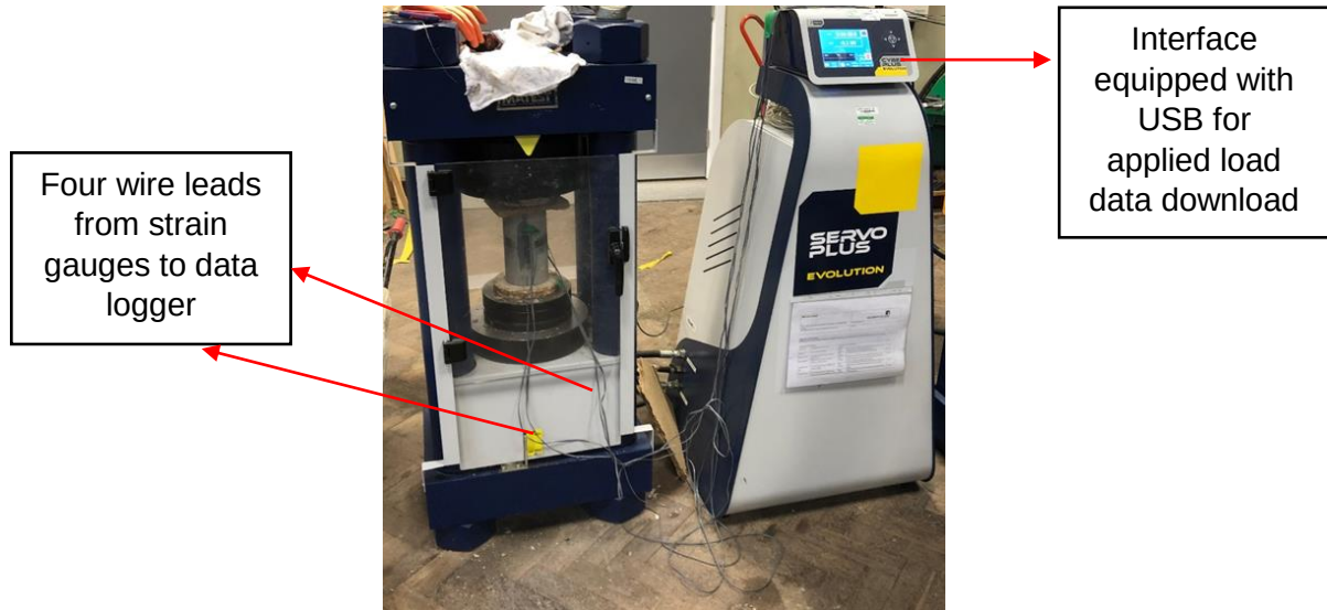
Figure 3.7: Photograph of Ø100 x 200mm cylinders subjected to incremental loads to failure
