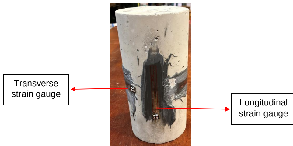
Figure 3.6: Photograph showing the strain gauge attached to a cylindrical specimen for static elastic modulus determination. Method adopted based on options recommended in ASTM C469/C469M-22 (160)
