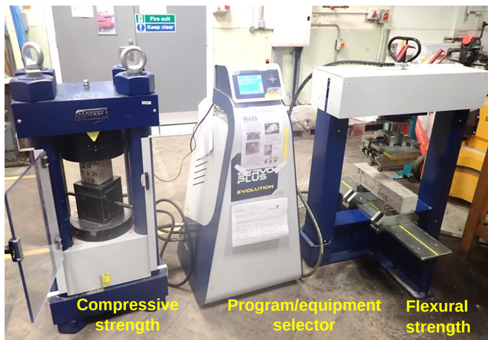
Figure 3.5: Photographs of the compressive and flexural strength testing equipment used in this study
