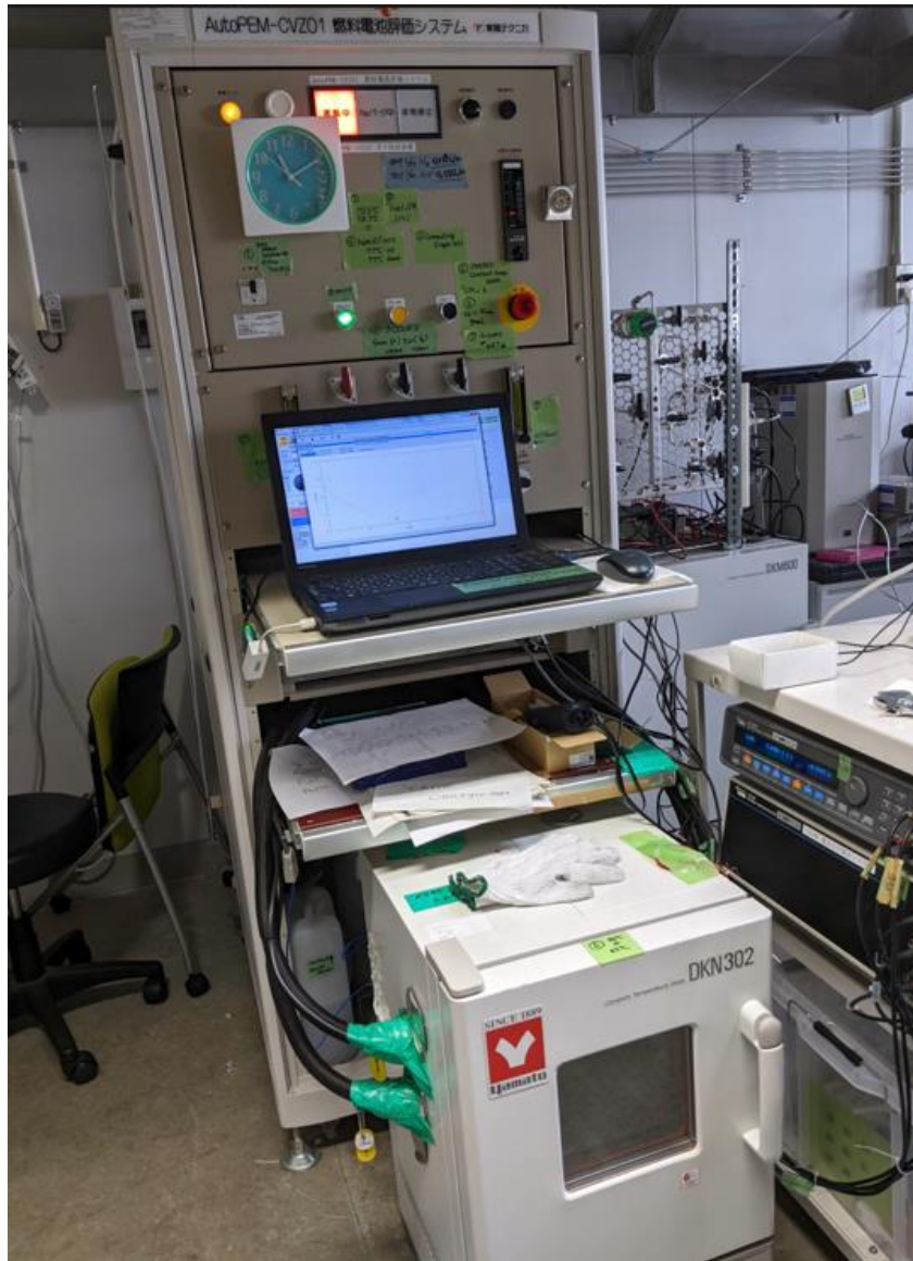
Figure D-14 Fuel cell test station with the constant temperature oven at the bottom of the picture.
