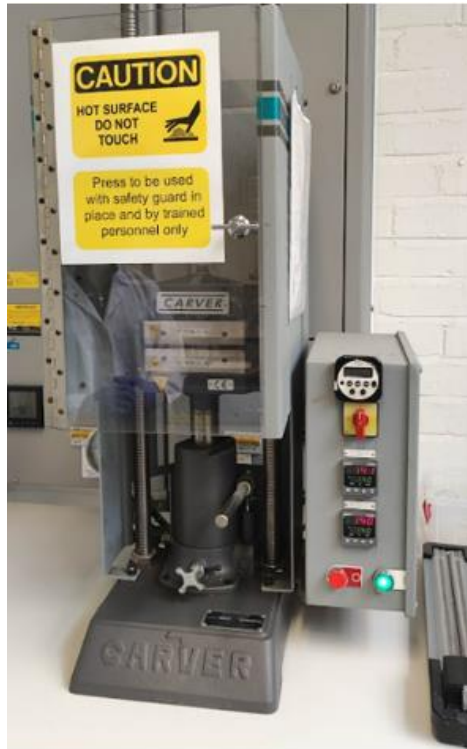
Figure D-5 Hot pressing of the MEA.
