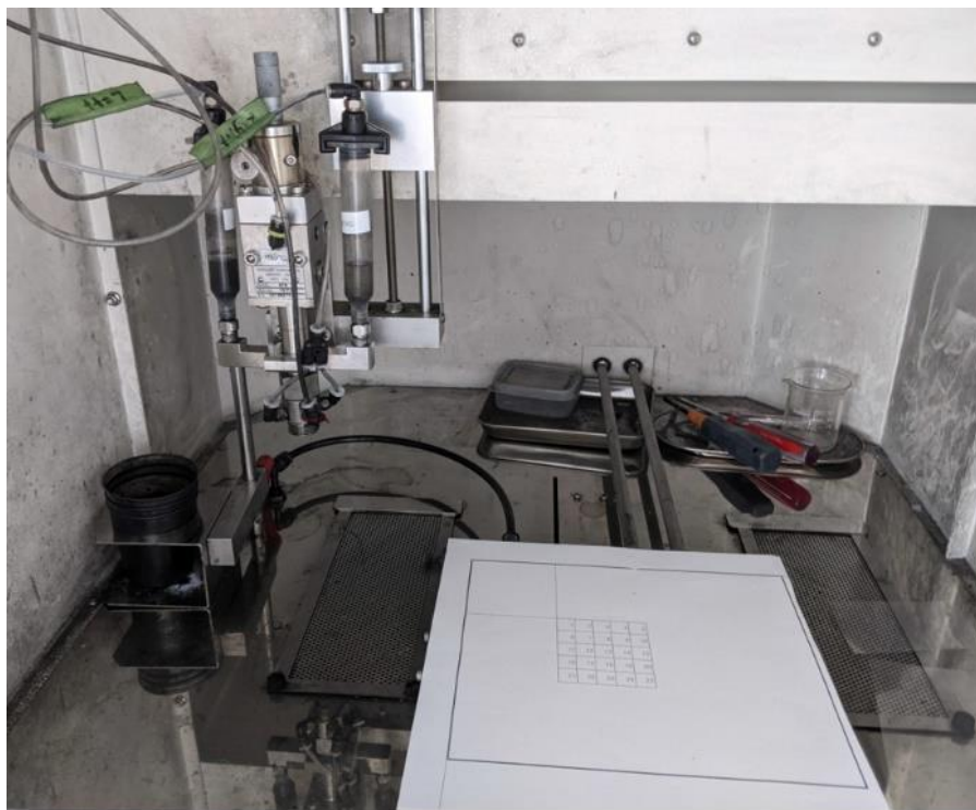
Figure D-11 Spraying machine with vacuum plate in the foreground.
