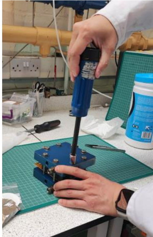
Figure D-7 Securing the fuel cell.
