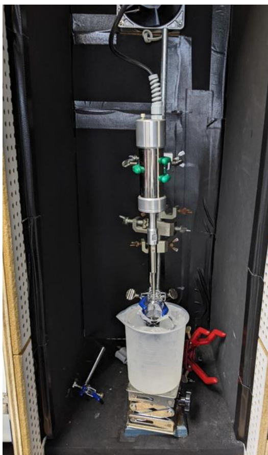
Figure D-10 Ink is placed into the sonic mixer for 30 minutes.
