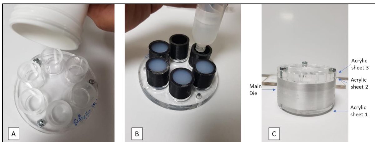
Fig.App 2: History of improvement for the compression specimens Moulds'. A) first trial, B) second trial, and C) third trial (optimum).
