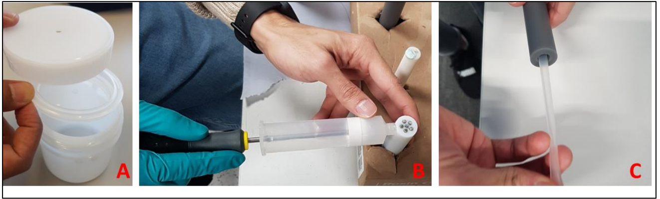
Figure 4-10: Fabrication process for soft component. A) a container covered with two lids for the pre-silicon mixing, each featuring a centrally located hole, B) injecting the pre-silicon into the augmented mould of Model-2, and C) the demoulding process, showing the extraction of a cured soft filament from its mould.
