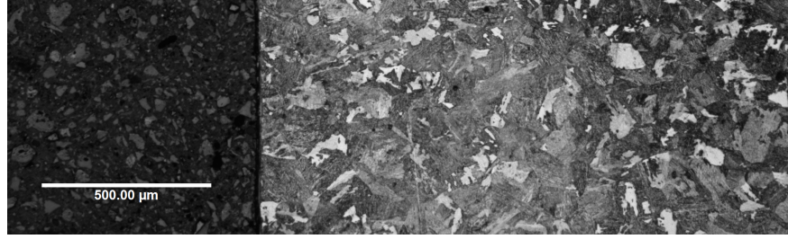
Figure 8.6: Optical micrograph of undeformed material for grain size measurement
