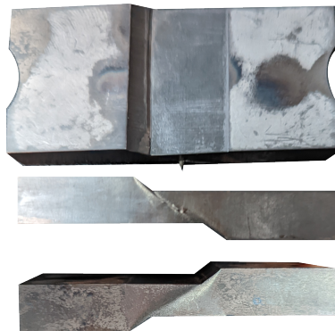
Figure 8.7: Post-deformation condition of two specimens deformed at 650°C
