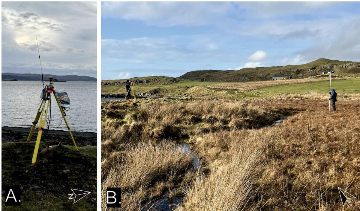
Figure 2.5. Photos of the dGPS setup and levelling techniques used at South Cuidrach. A. Temporary benchmark (TBM) site and Leica System 500 dGPS setup. B. The theodolite level used to survey features from TBM.
