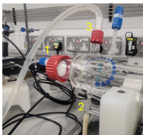
Figure 14: a) Labelled picture of the small flow reactor set up for the variable flows method. 2 stirrer plates are shown (grey boxes with blue dials); during experiments, a third stirrer plate was also present. b) Close up of inlet, with components numbered; 1. gas inlet line 2. liquid inlet line 3. water jacket connection to recirculating water bath. c) Close up of outlet with components numbered 1. gas outlet line 2. liquid outlet line 3. water jacket connection to recirculating water bath 4. additional line used for cleaning, which was not present during experiments (the glass port was capped).
