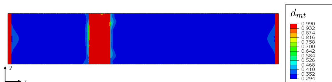
Figure 4.5: Matrix tensile damage in the 90° specimen
