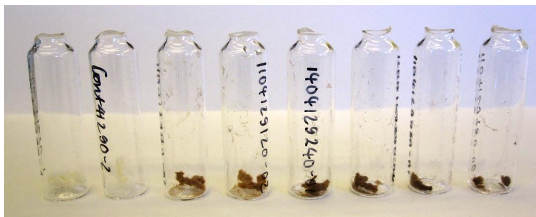
Figure 4.2. Isothermally heated undyed textile samples after heating at 110°C and drying. Left to right: controls (2 x), 120 h (2 x), 240 h (2 x) and 480 h (2 x) time points.
