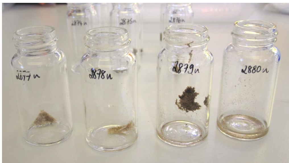
Figure 4.1. Undyed samples buried at Lejre, during washing. Left to right: buried 1, 2, 4 and 8 years.
