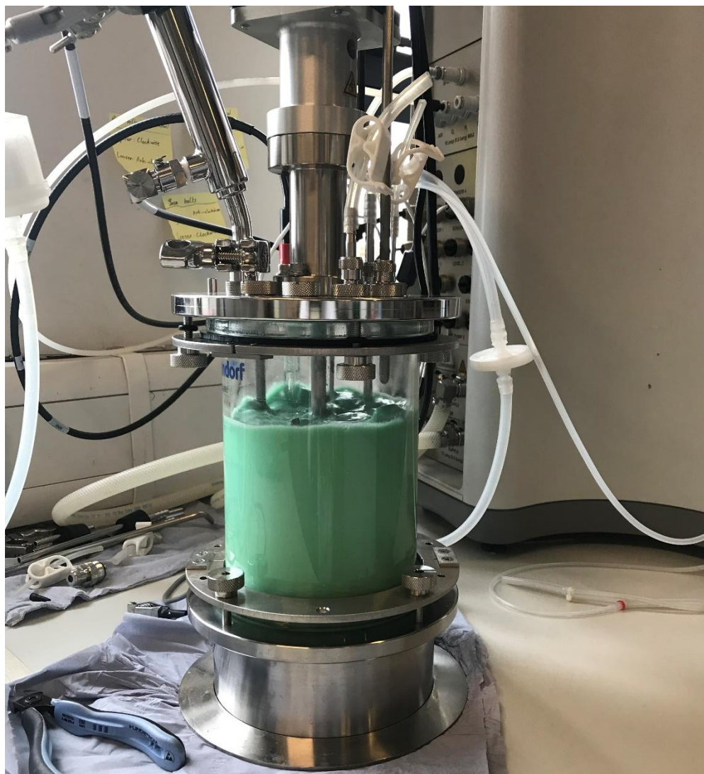
Figure 5.1: STR set-up containing a precursor solution of nickel sulphate, ammonia and sodium hydroxide.
