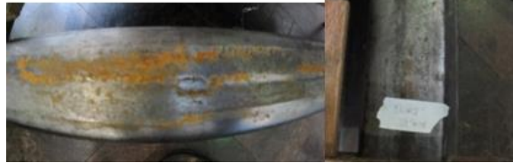
Figure 6. 14: Example of railhead images for rust day2. Horizontal with camera-railhead distance \approx 300\text{mm} distance (L) and vertical with camera-railhead distance \approx 700\text{mm} (R) (21-04-22)
