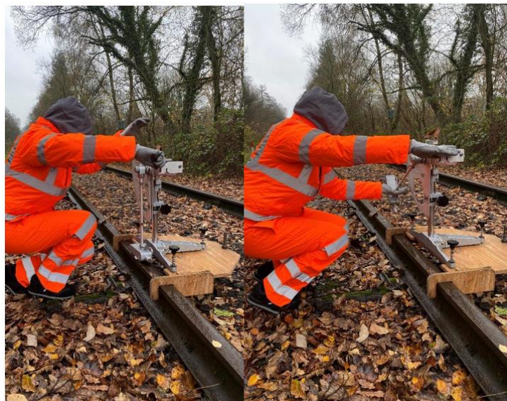
Figure 4. 5: Pendulum arm head striking the railhead (left) and pendulum arm caught before return (right)
