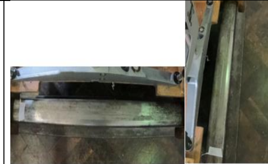
Figure 6. 7: Example of railhead images for cleaned with wire brush. Horizontal with camera-railhead distance \approx 1450\text{mm} (L) and vertical with camera-railhead distance \approx 1450\text{mm} (R) (13-04-22)
