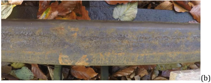
Figure 4. 9: (a) \mu against relative humidity with a colour map representing railhead temperature for Wirksworth (left) and Idridgehay (right) on 13-11-2020 and (b) Railhead image with visible oxidisation with \mu of 0.33 from Wirksworth on 13-11-2020
