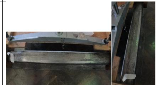
Figure 6. 10: Example of railhead images for 1st water spray. Horizontal with camera-railhead distance \approx 1450\text{mm} distance (L) and vertical with camera-railhead distance \approx 1450\text{mm} (R) (13-04-22)
