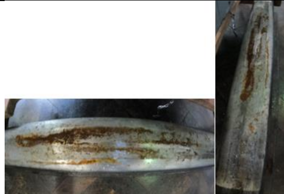
Figure 6. 24: Example of railhead images for rust day5 + reduced water spray. Horizontal with camera-railhead distance \approx 450\text{mm} (L) and vertical with camera-railhead distance \approx 1000\text{mm} (R) (10-05-22)
