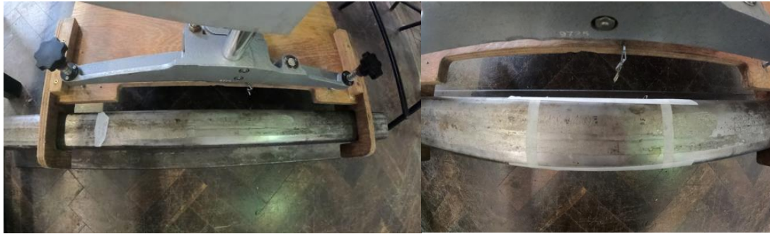
Figure 6. 3: Railhead image taken at a height of 1450mm (L), and the distance used for the prediction tool training (between 400mm-500mm from the railhead position) (R)
