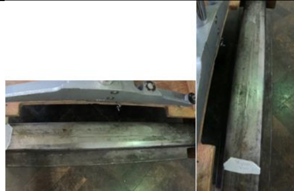
Figure 6. 6: Example of railhead images for cleaned with alcohol wipe. Horizontal with camera-railhead distance \approx 500\text{mm} (L) and vertical with camera-railhead distance \approx 900\text{mm} (R) (13-04-22)
