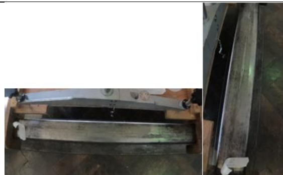
Figure 6. 9: Example of railhead images for previous day wet. Horizontal with camera-railhead distance \approx 1450\text{mm} (L) and vertical with camera-railhead distance \approx 1450\text{mm} (R) (13-04-22)
