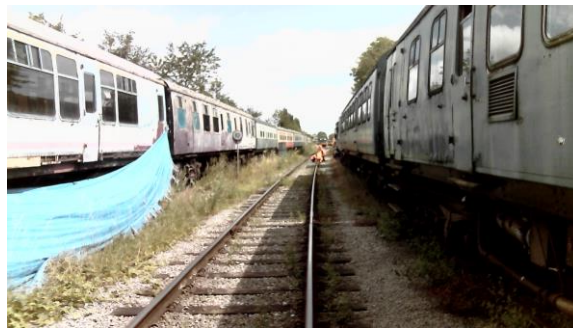
Figure 7. 27: Forward facing image of a hot spot recorded with air temperature 28.7^{\circ}\text{C} with a shaded railhead section recording 21.1^{\circ}\text{C} on the railhead IR sensor
