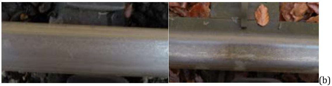
Figure 4. 8: (a) \mu against relative humidity with a colour map representing railhead temperature for Wirksworth on 21-11-2019 and (b) Dry railhead (left) and damp railhead (right) from Wirksworth on 21-11-2019
