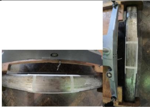
Figure 6. 5: Example of railhead images for uncleaned state. Horizontal with camera-railhead distance \approx 450\text{mm} distance (L) and vertical with camera-railhead distance \approx 1450\text{mm} (R) (13-04-22)
