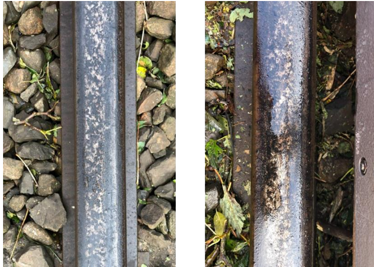
Figure 5. 12: Sample of railhead contamination recorded at the Salisbury 2021 incident
