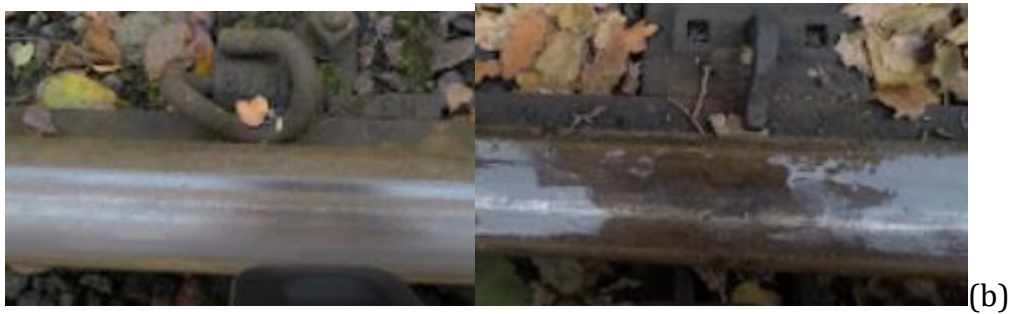
Figure 4. 7: (a) Plot of \mu against relative humidity with a colour map representing railhead temperature for Idridgehay on 21-11-2019 and (b) Shaded dry railhead (left) and artificially wetted railhead (right) at Idridgehay 21-11-2019
