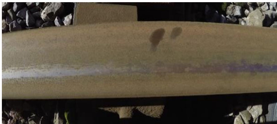
Figure 4. 12: (a) \mu against relative humidity with a colour map representing railhead temperature for Darley Dale on 02-10-2019; (b) Corresponding railhead image for the Darley Dale \mu of 0.13
