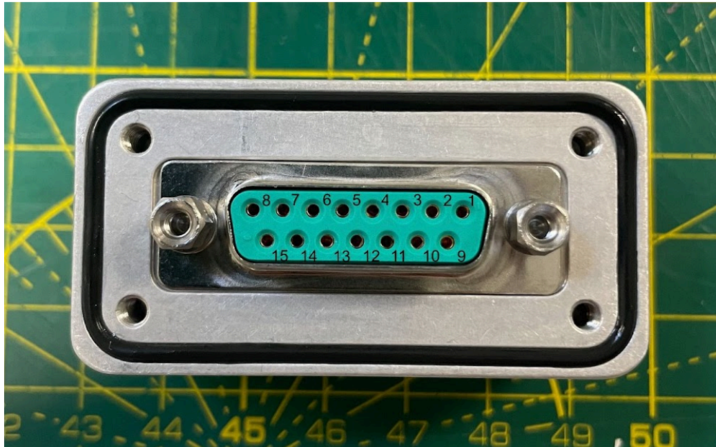
Figure 3.10: 15-pin passthrough connector viewed from the internal side. The rubber O-ring can be seen which creates the airtight seal. The metal exterior that provided the hermetic seal for the connector was produced by the York University Machine Workshop.
