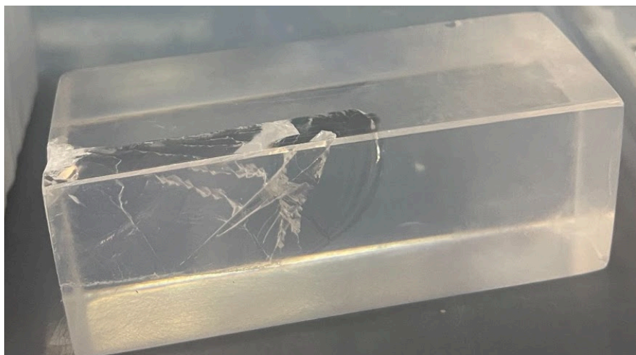
Figure 3.2: Crystal 2 in the glove box after an incident that caused damage to it and Crystal 4. Large cracks can be seen in the upper left quadrant.
