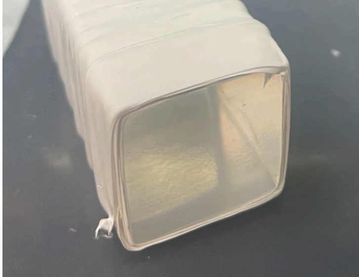
Figure 3.3: Crystal 4 wrapped on the sides with PTFE tape and the end cap removed. A small crack can be seen in the top right corner of the end face.
