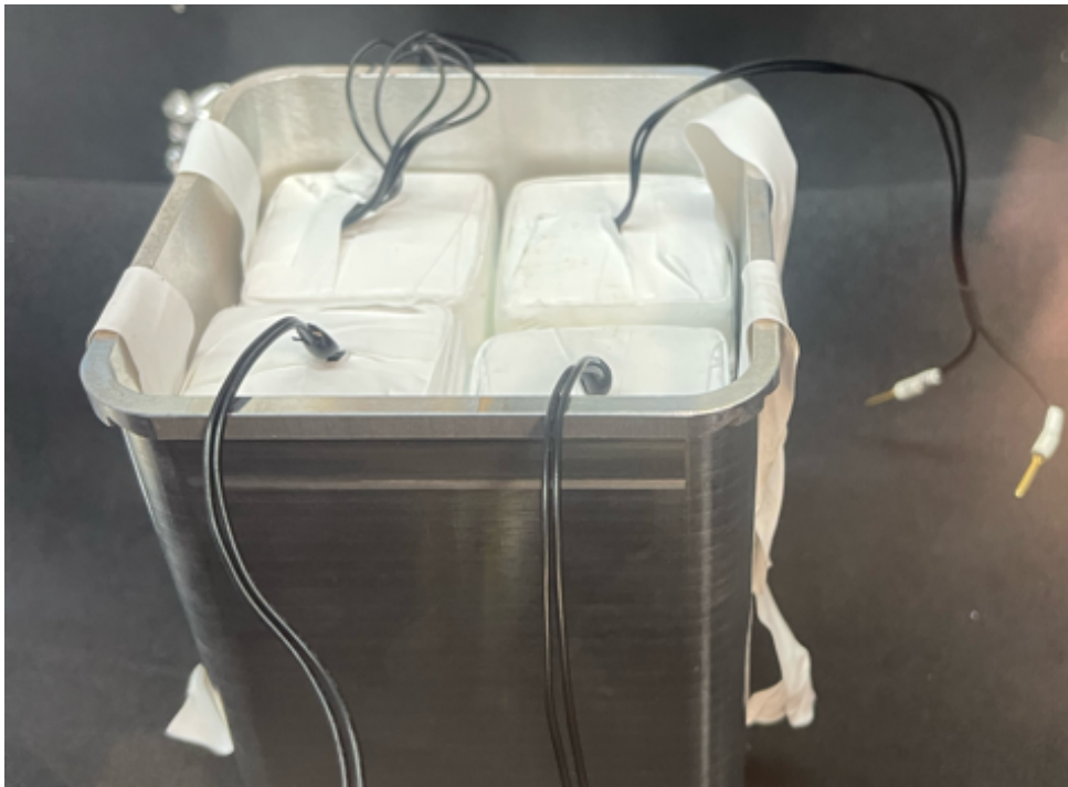
Figure 3.11: Wrapped crystal placed inside the aluminium housing before being wired to the connector and hermetically sealed. Strands of PTFE can be seen looped underneath the crystals for easier extraction.
