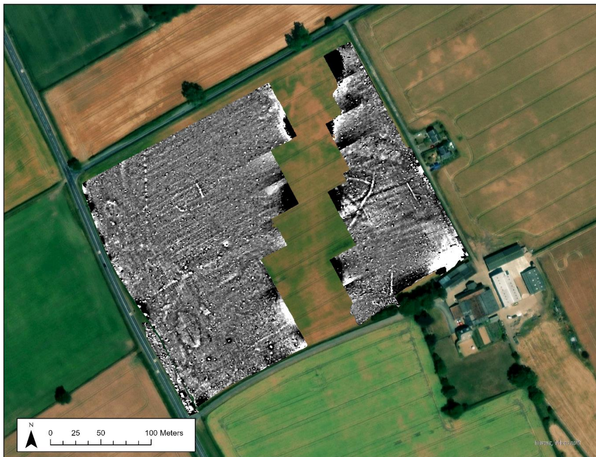
Figure 6.25 Survey area H Magnetometry greyscale. The route of a high-pressure gas main can be seen cutting north-south across the survey area.
