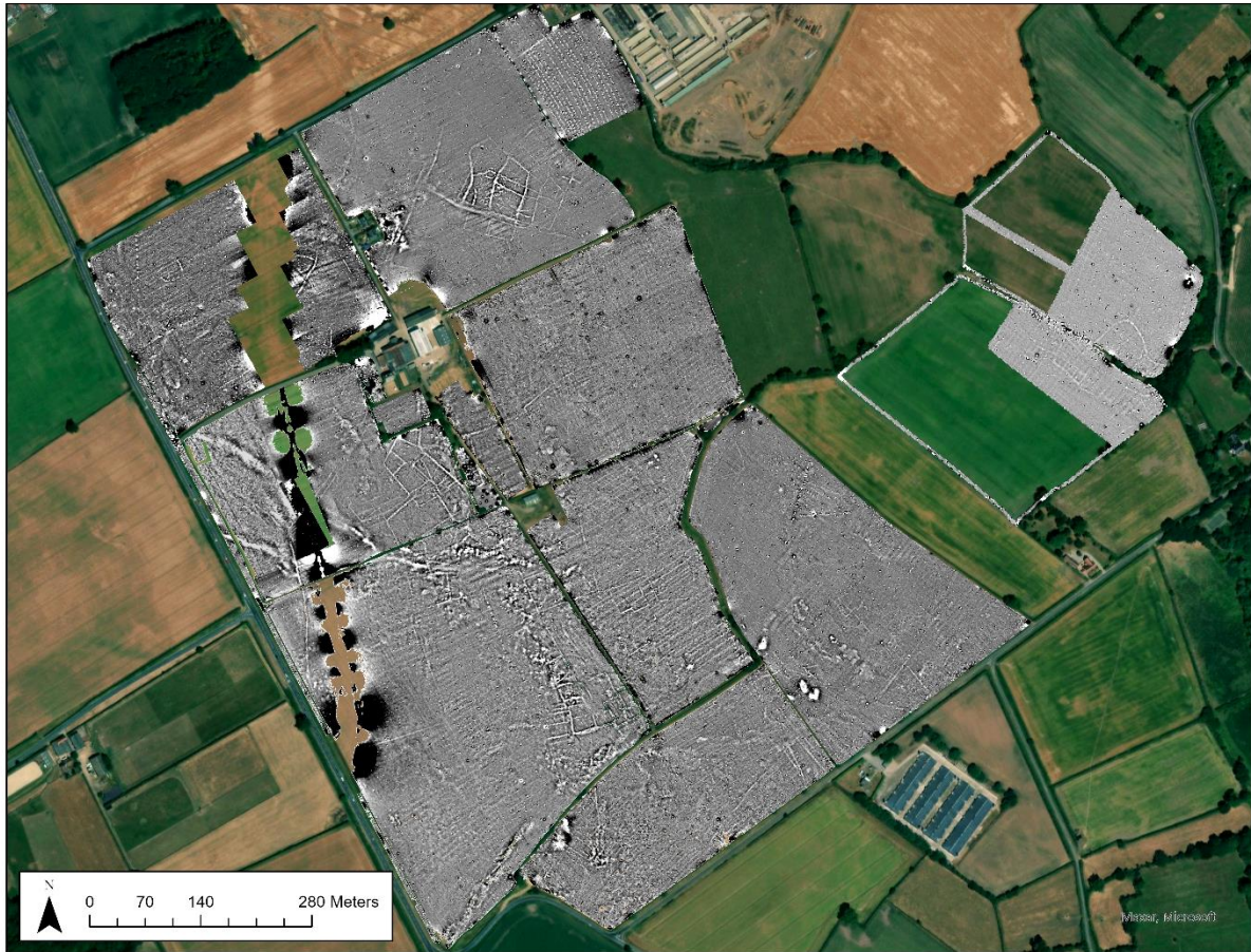
Figure 6.5 All Survey Greyscale. Note the data gaps related to the gas pipeline (trending SW to NE across the eastern side of the site) as well as along field boundaries.
