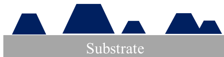
Figure 20 VW growth with 3D islands of deposited material atop the substrate.
