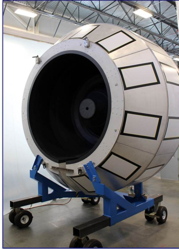
Figure 4.16: The fully assembled High Threshold Cherenkov Counter, taken from Ref. [79].
