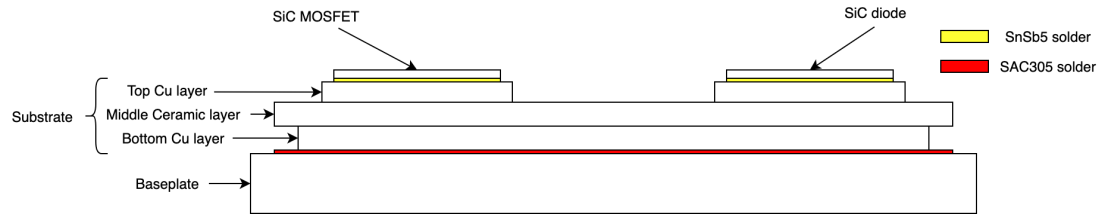
Fig.1-7 Cross sectional diagram of a typical SiC power module
