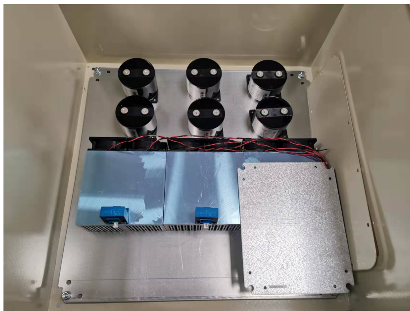
Fig.4-7 Capacitors, heatsinks, and sensors mounting
