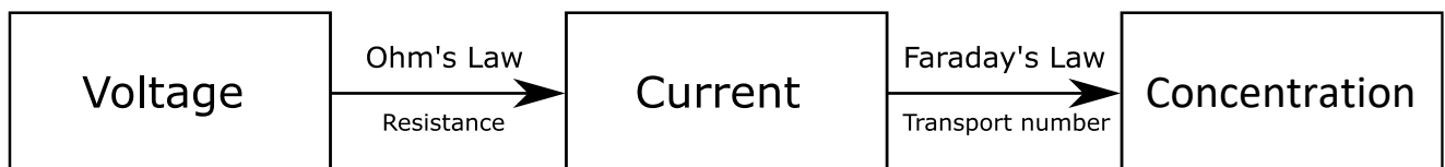
Figure 2.4: A schematic representation of an overview of most circuit-based models. Known/measured variables are in boxes and the links between them are shown with the arrows. This demonstrates how virtually any model deficiency can be accounted for through modifications to the electrical resistance and membrane transport number.
