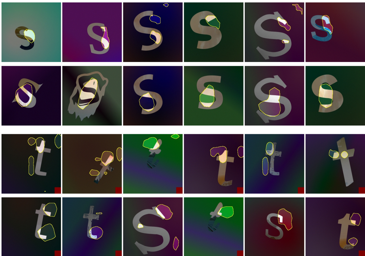
Figure 4.4: The top six training images for which four kernels in the second convolutional layer of AlexNet most strongly activate, with the corresponding dissection maps. All four kernels show strongest activation for regions overlapping with the core feature, the character mask. The bottom two rows show image samples for the latter two kernels which also are from the majority group, with the spurious bias feature in the corner, yet the kernels in question do not strongly activate to the bias. In these cases, the kernels pay more attention to the characters.
