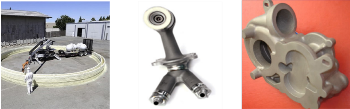
Figure 2.4.: A) Digital Building Platform design at MIT [22], B) Fuel nozzle of Aeroplane produced by AM[24], C) Water pump for a car produced by SLM [25].
