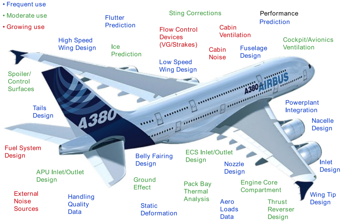
Figure 1.1: Graphical representation of how “CFD moved from an exploratory tool to a full flight physics production” in Airbus aircraft design cycle, image for CFD application in 2010, and quote from the company’s head of aerodynamic research and technology, [2].
