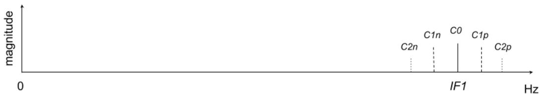
Figure 21. An RX TMA (e.g. STMA) converts from a carrier ( $C0$  boresight beam at carrier) to a set of harmonic beams, each centred at an angle of arrival for that beam.
