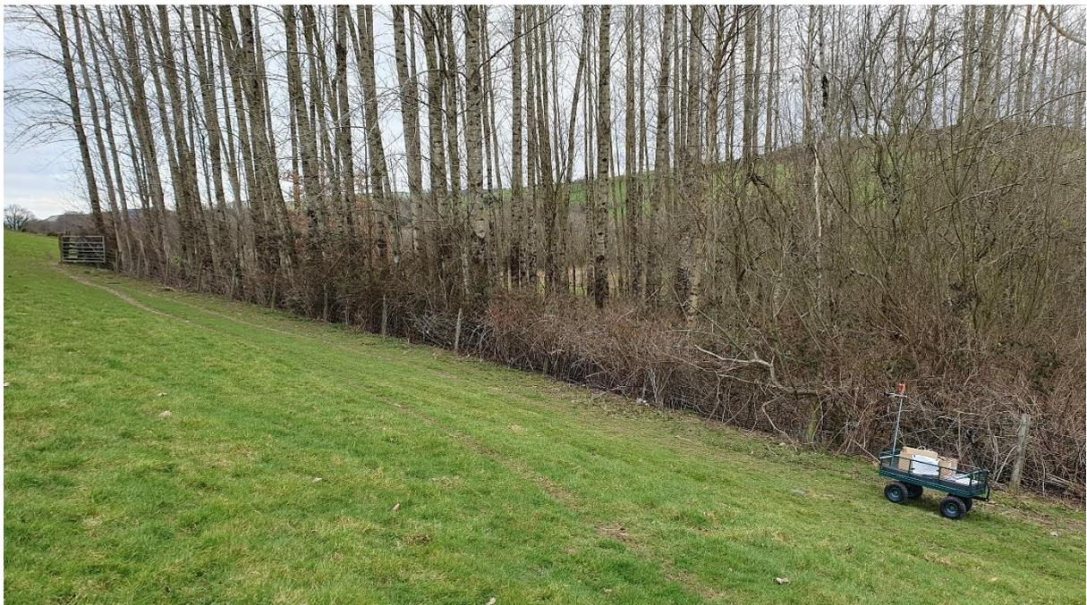
*Figure 17. Propagation through a wooded scrub area (route N) – TX site. RX system is on the other side of wood. Both TX and RX start near the gate on the left and are moved away from each other to increase the path length through the wood.*
