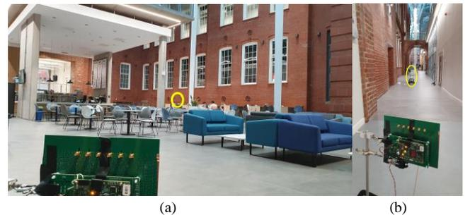
Fig. 9. TMA TX propagation field test: (a) TX in café area, RX by rear wall (ringed), (b) Corridor test area: view from behind TMA towards RX (ringed).
