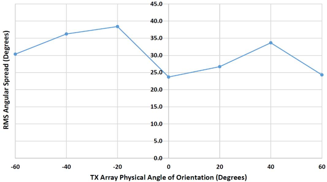
Figure 38. Calculated RMS AS for Café scenario (TX array rotated in steps for each TMA run, constant distance to RX).
