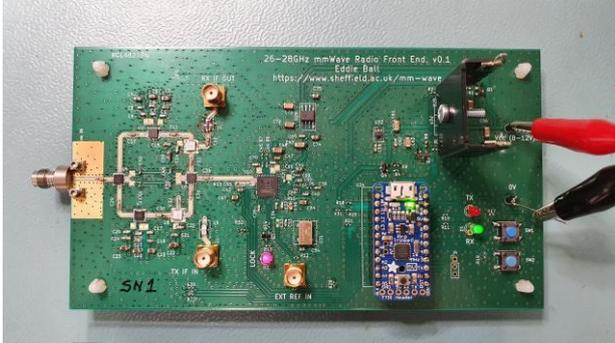
Fig. 2. Fully assembled 28 GHz RF frontend PCB.
