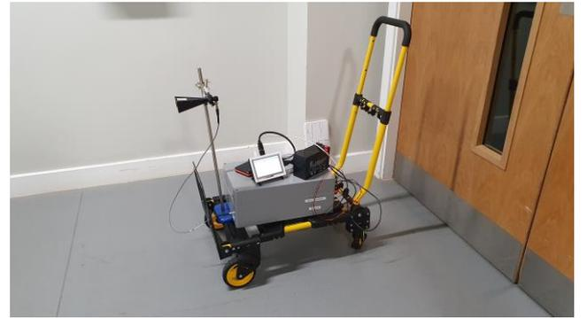
Fig. 10. TX system during indoor soundings at The University of Sheffield.
