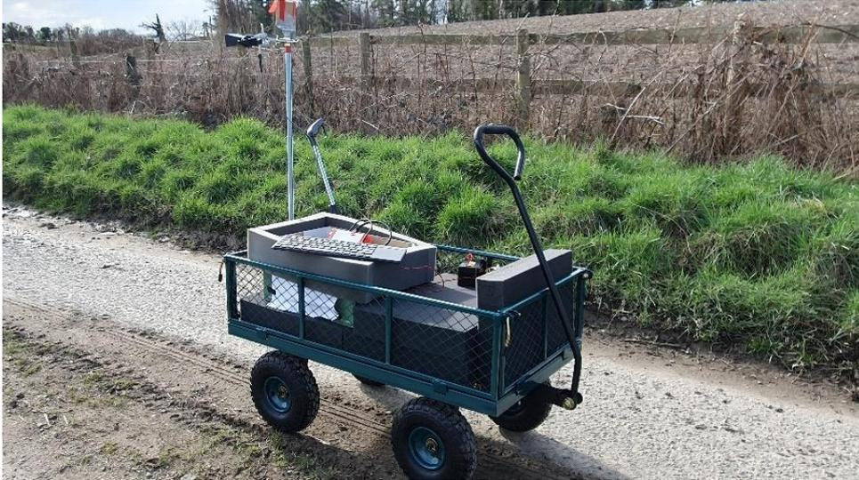
Figure 10. One of the sounder systems in a cart (route A). The 28 GHz horn antenna can be seen in stand on left of cart.
