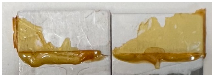
Figure 4. 15: Photo to show the cohesive failure during the lap shear test of P(DCPD-ENB-IBMA-NBMMA)
