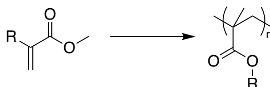
Scheme 1. 2: polymerisation of a methacrylate monomer to a poly(methacrylate)
