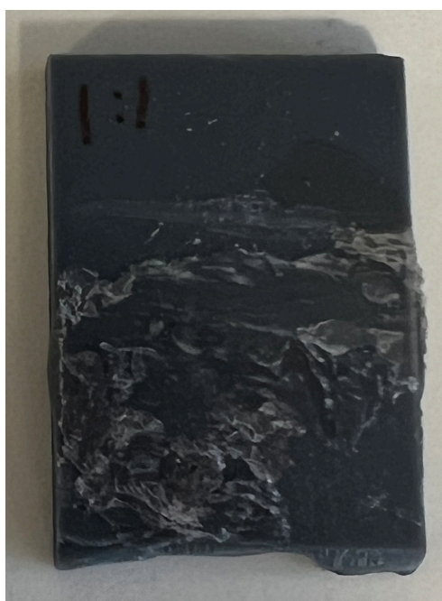
Figure 3. 20: Photo of PVC compressive lap shear after testing with 1:1 P(NBMMA-co-NBCA)
