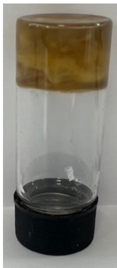
Figure 3. 8: Photo to show that MMA monomer had polymerised due to residual Ru catalyst.
