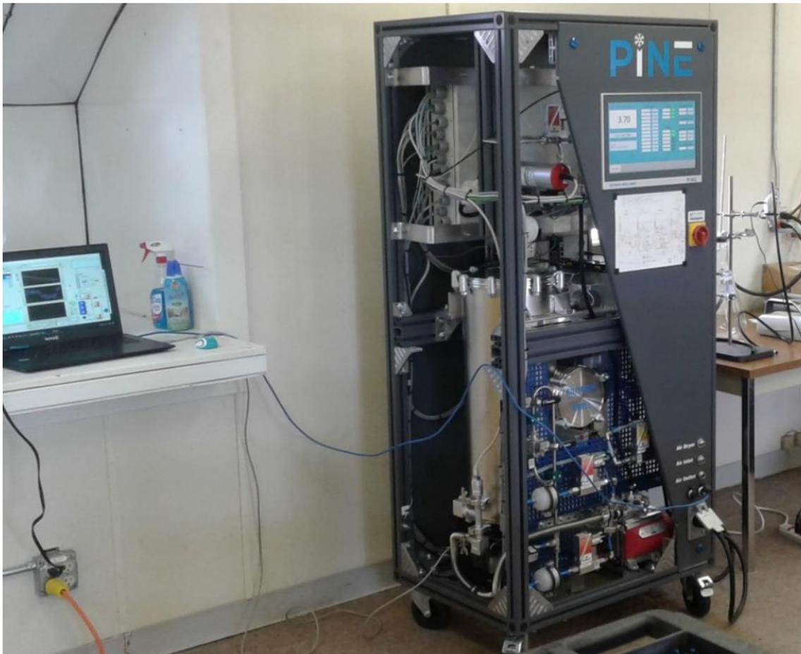
**Figure 1.11:** Photograph of a commercial PINE instrument making continuous INP measurements in Oklahoma. Side panels are removed to show the internal workings of the PINE. Figure A7 from Möhler et al. (2021).
