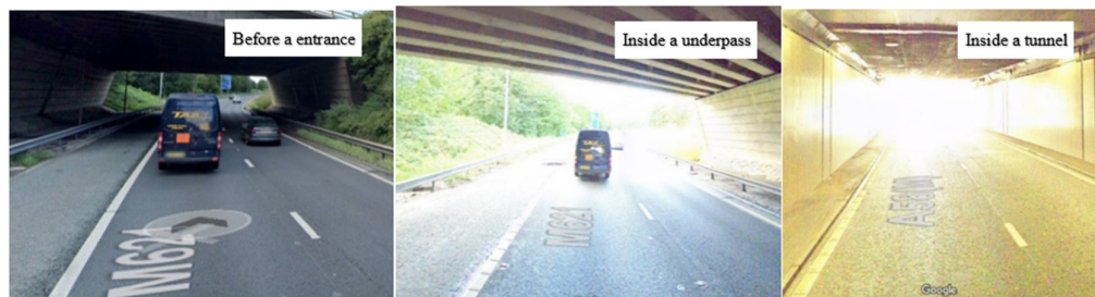
Figure 2.8 An example of the limitation in vision-based systems on near the exit of the underpasses and tunnels (Google Street View).
