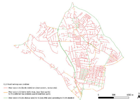
C3,3 Road marking wear condition
