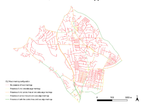
C3,2 Road marking configuration
