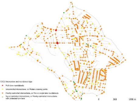
C15,1 Intersection and roundabout type
