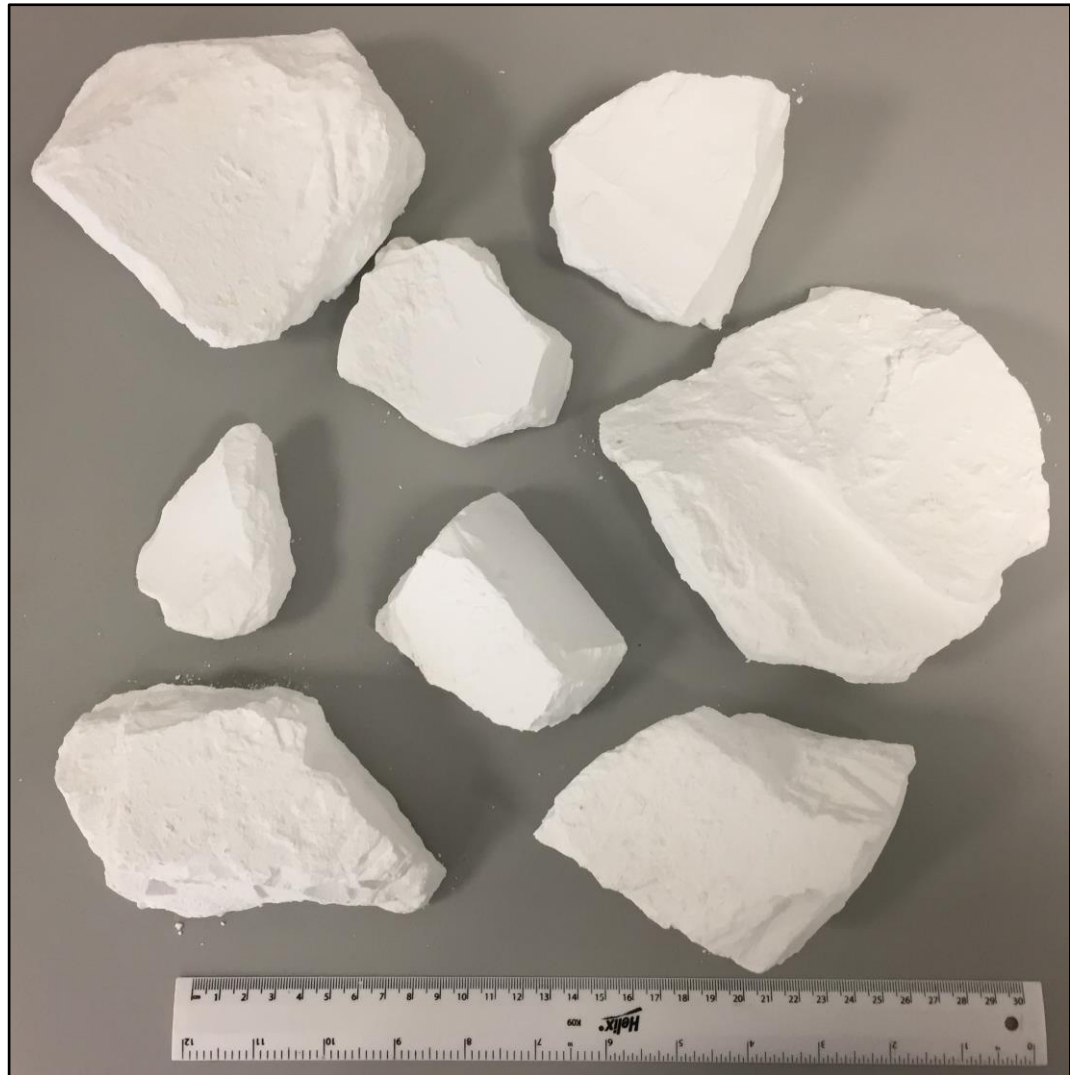
Figure 1.4 - Some debris collected from the spray drier bend. Note – samples of the debris were received at Leeds and the materials were examined. During this examination, the photo shown was taken.
