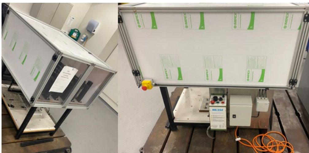
Figure 6.2 The current status of the fatigue rig after the addition of the protective guard, and reassembly.
