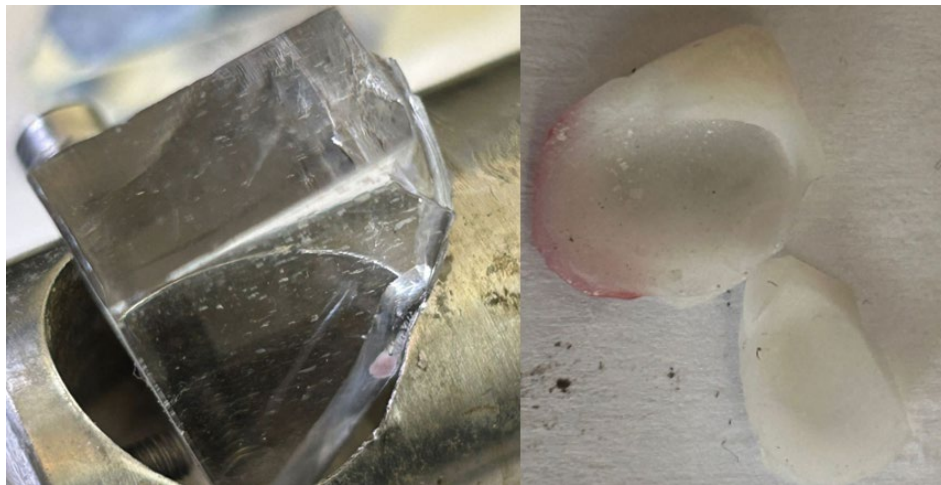
Figure 6.8 PMMA material not damaged due to its thickness, whereas a ceramic type restoration is fractured under cyclic impact.
