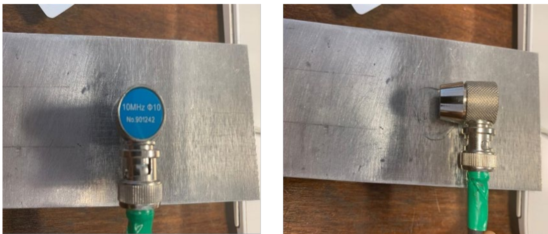
Figure 4.4 10 MHz commercial transducers on aluminium bar.
