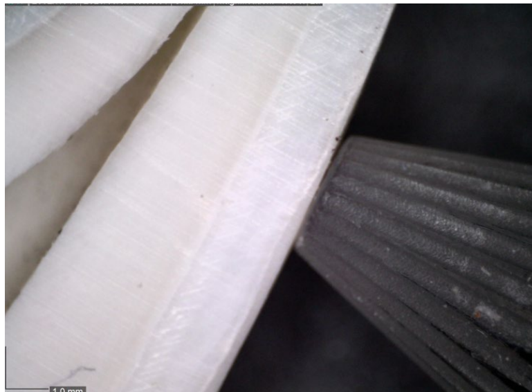
Figure 5.14 Tooth number 7 Sensor delay line in contact with enamel side of right section of a central incisor.
