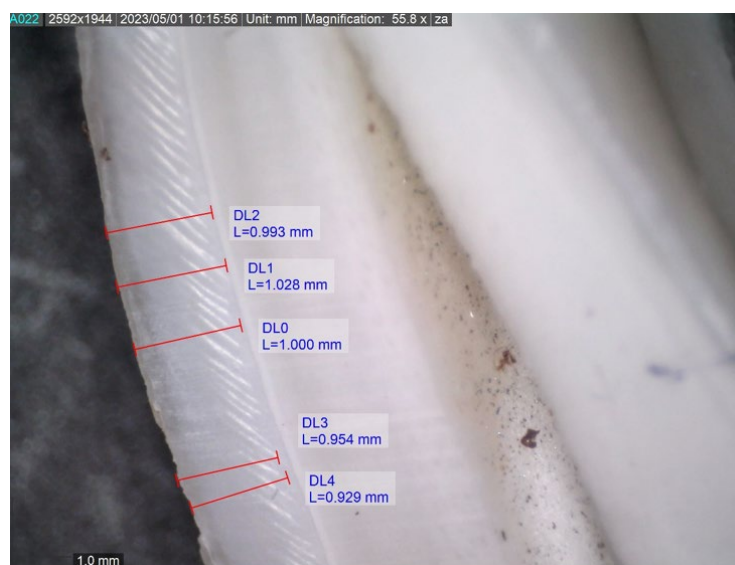
Figure 5.12 Measurement of enamel structure thickness in different spots using a digital microscope (some inaccuracy with the lines).
