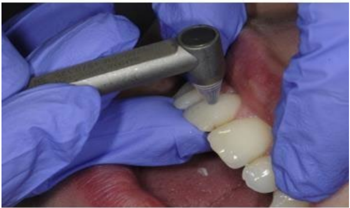
Figure 2.10 Ultrasonic transducer position on teeth when taking measurements (74).
