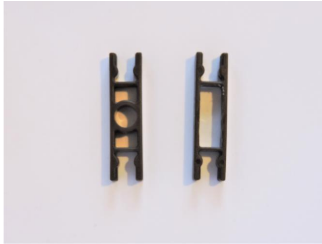
Figure C.2: An unmodified K'NEX two-way connector (left), next to a modified K'NEX two-way connector (right)
