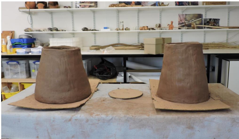
Figure E.4: The fully-built clay stoves
