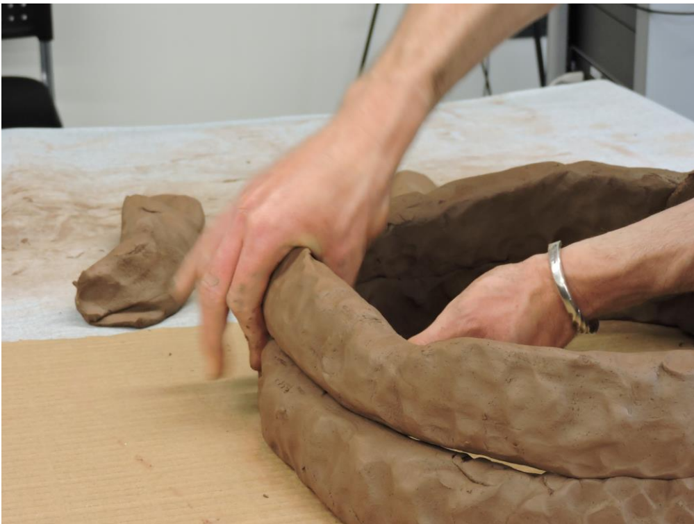
Figure E.2: Clay coils being stacked and pinched together
