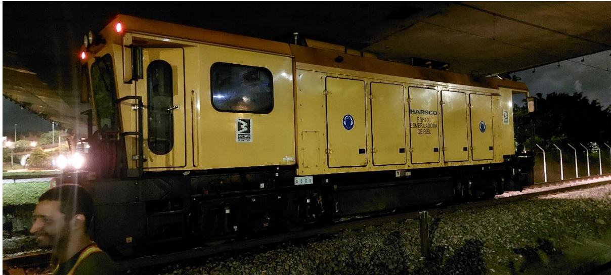
Figure 31: The Harsco RGH10C rail grinder employed for the grinding operation in Medellín Colombia
