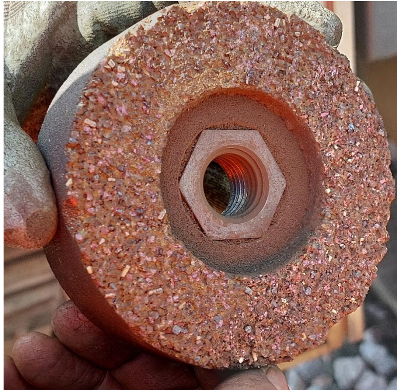
Figure 46: Condition of a used face grinding wheel at end-of-use for the rail grinding operation at Drax Power Station.
