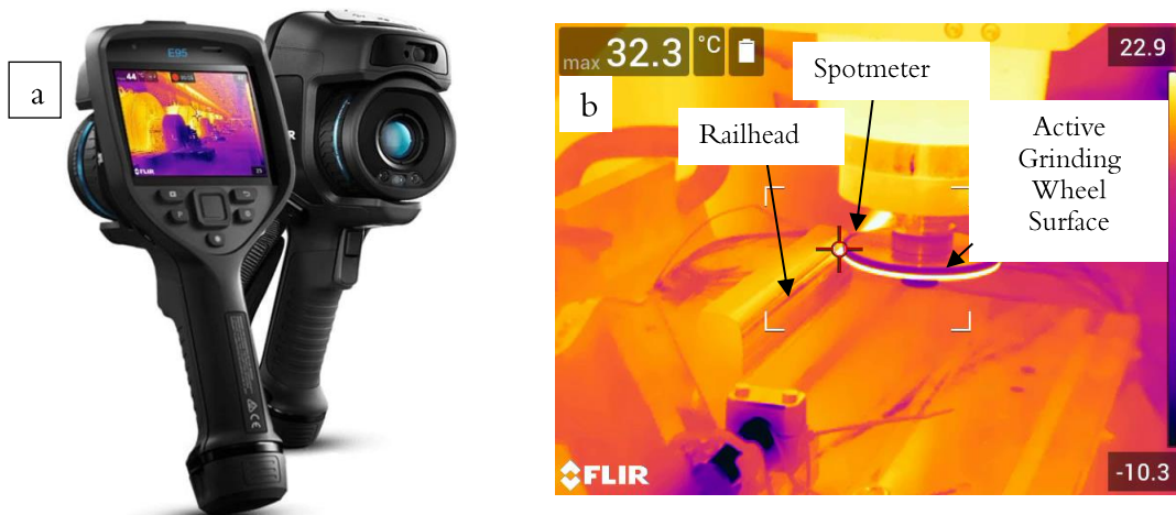
Figure 57: (a) FLIR E-95 thermal camera and (b) corresponding thermal image obtained in its use during a grinding pass
