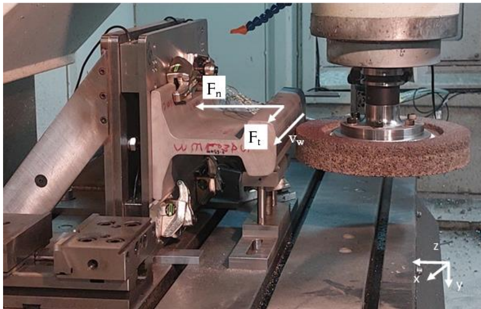
Figure 125: The orientation of the component grinding forces F_n and F_t which act on the rail and grinding wheel interface during a peripheral grinding pass.
