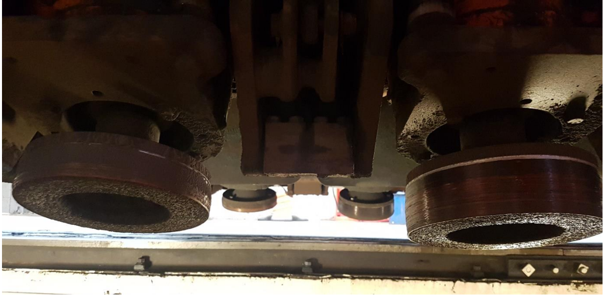
Figure 4: An assembly of abrasive \text{AlO}_x grinding wheels at various stages of use beneath a grinding train.
