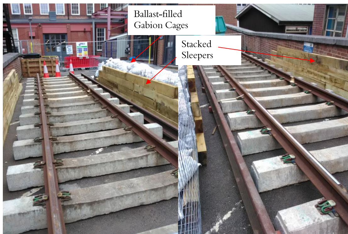
Figure 141: The track panel set-up developed for the use of the grinding trolley.
