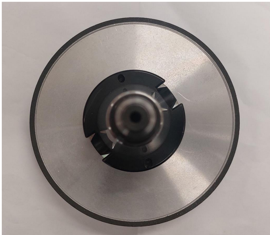
Figure 56: Electroplated CBN grinding wheel utilised in grinding trials.
