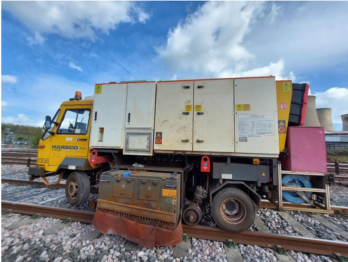
Figure 44: The Harsco Möser Road/Rail Grinder (RO-V149) used in grinding operations at the Drax Power Station
