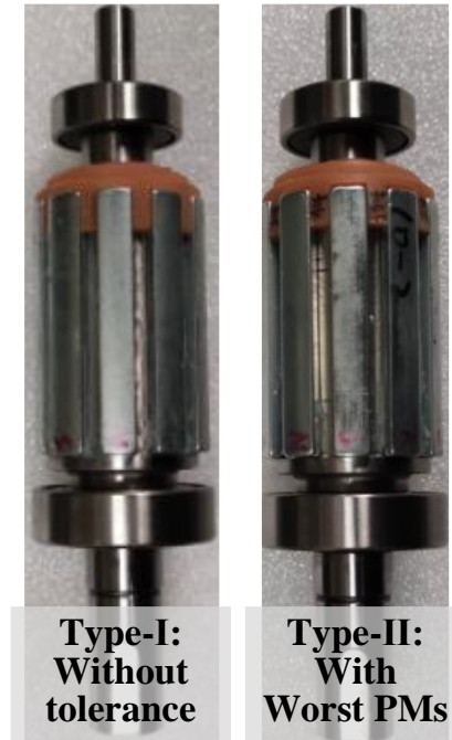
(b) Rotor (Type-I: without tolerance, Type-II: with Worst PMs)
