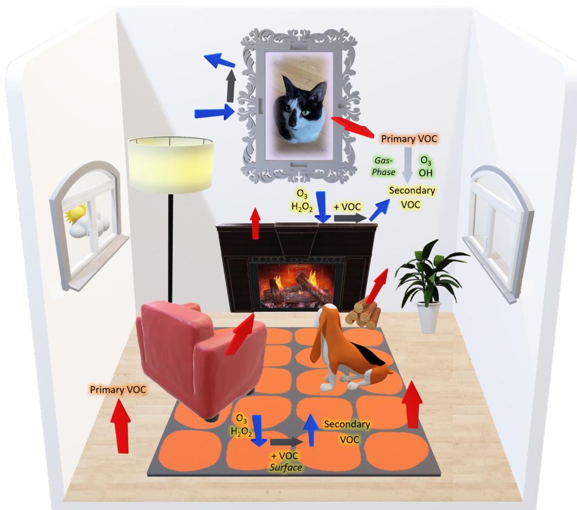
Figure 4.1: The chemical processes and transformations following deposition of oxidants on internal surfaces in the indoor environment.
