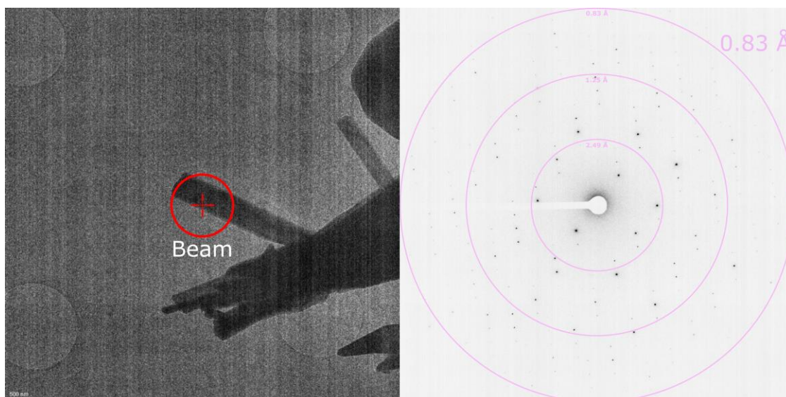
Figure 5.5. Example Compound 5.1 crystal and diffraction pattern. Left: TEM brightfield image of Compound 5.1 crystal, red circle represents the beam diameter ( 1.05\ \mu\text{m} ). Right: Representative electron diffraction pattern, with resolution rings. Outer resolution ring is 0.83\ \text{\AA} .
