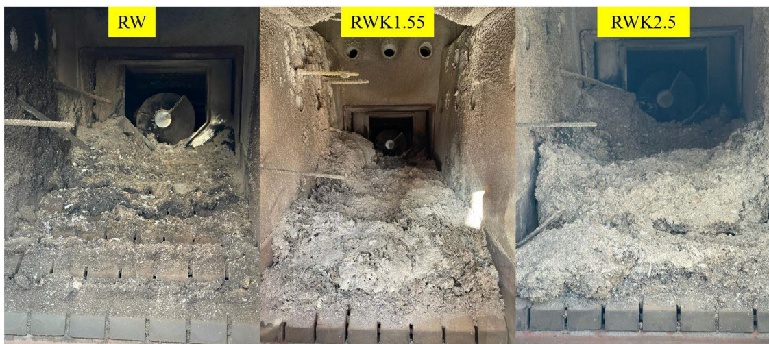
Figure 5-8 The post-firing condition on top of the bed of the moving grate for recycled wood (RW) with kaolin addition at 1.55% (RWK1.55) and 2.5% (RWK2.5).
