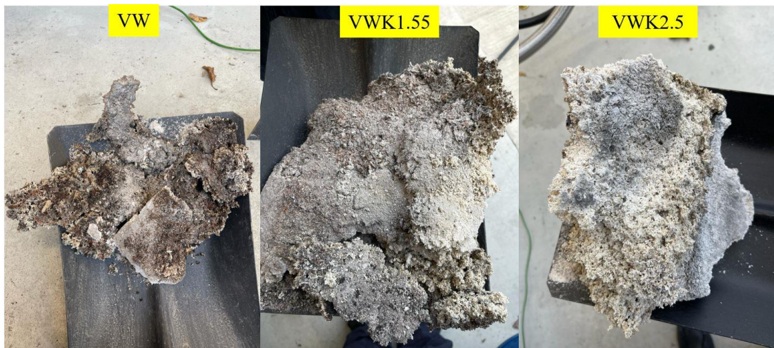
Figure 5-7 Slag formation byproducts of firing for virgin wood and mixtures of kaolin.
