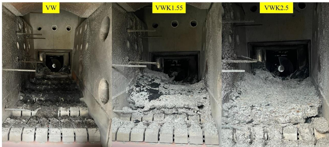
Figure 5-6 The post-firing condition on top of the bed of the moving grate for virgin wood (VW) with kaolin addition at 1.55% (VWK1.55) and 2.5% (VWK2.5).
