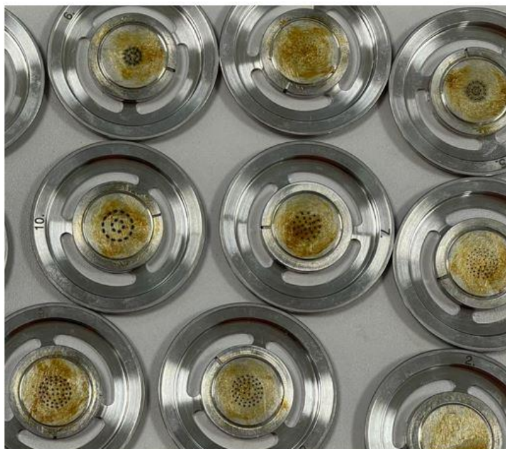
Figure 2-13 Ultrafine fly ash samples on polycarbonate foil with apiezon-H grease.
