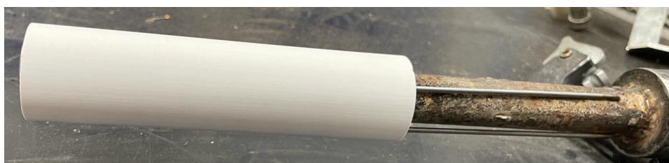
Figure 2-10 A ceramic coupon is installed at the tip of the stainless-steel probe.
