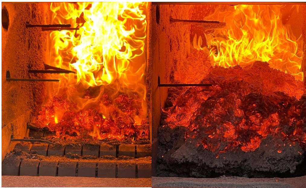
Figure 5-5 Severe agglomeration of the recycled woods with addition of kaolin during firing. Left: without kaolin, right: with kaolin.
