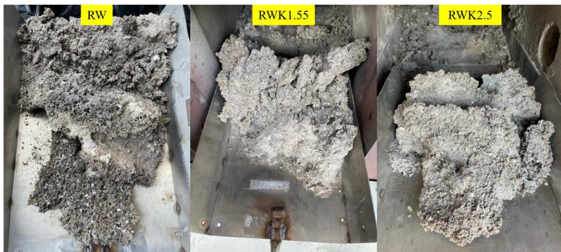
Figure 5-9 Slag formation byproducts of firing for recycled wood and mixtures of kaolin.
