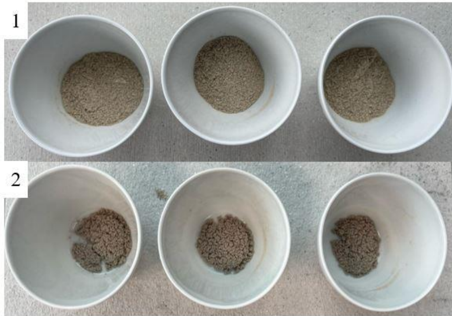
Figure 2-15 Representative sample of ash in the crucible for moisture and ash content analysis. Top image (1): Ash before firing in the muffle furnace. Bottom image (2): Ash after firing in the muffle furnace.
