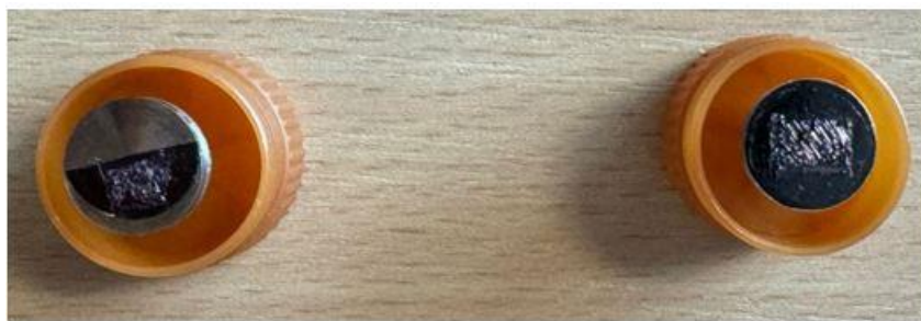
Figure 2-25 Specimen samples of ultrafine fly ash (<10µm) with gold coating for SEM-EDS analysis.
