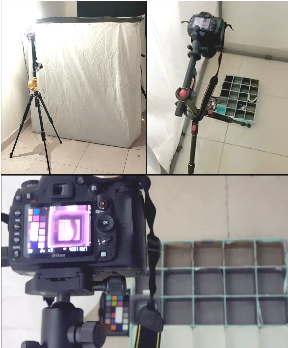
Figure S3.6: A collection of images illustrating the photography setup for Chapters 3 and 4. The top left image shows the EyeColor Arc MT70D lamp next to the custom-built tent. The images of the top right and bottom show the Nikon camera over the photography containers.
