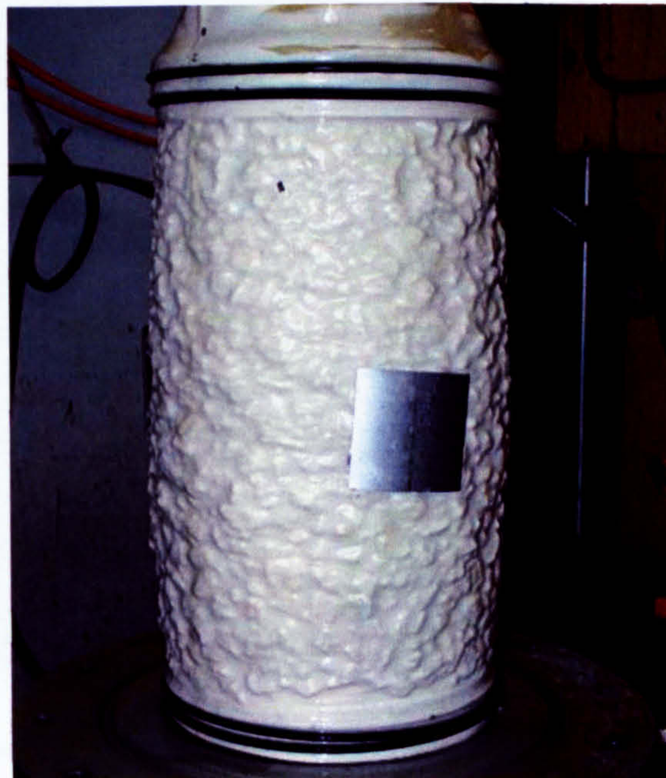
Plate 3.2 - Showing a target on the side of the specimen and bulging failure after a monotonic load triaxial test
