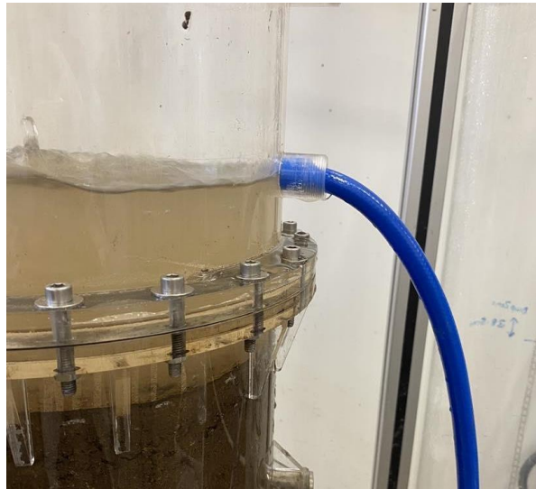
Figure 57. Port used to allow flow of excess water to maintain a constant head/depth.
