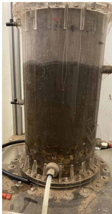
Figure 60. Soil column being saturated with water, using the bottom-most port. Note visible 'water-line' indicating level of saturation.
