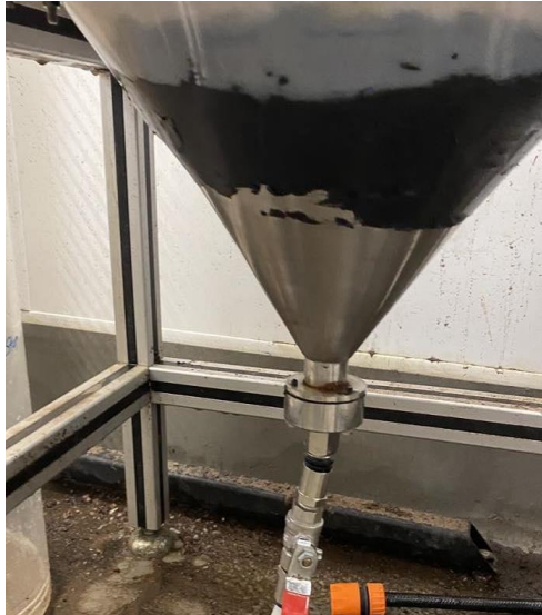
Figure 55. Funnel at bottom of column with tap attached. Pipe leads into lab floor drain.
