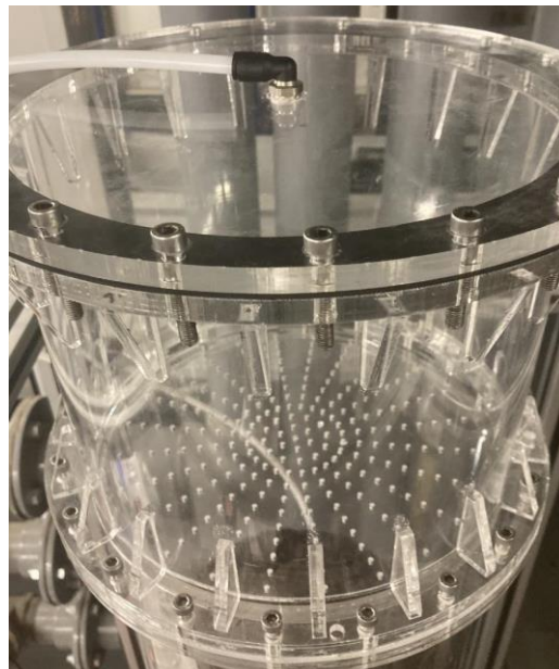
Figure 56. Shower head plate fitted at top of column.
