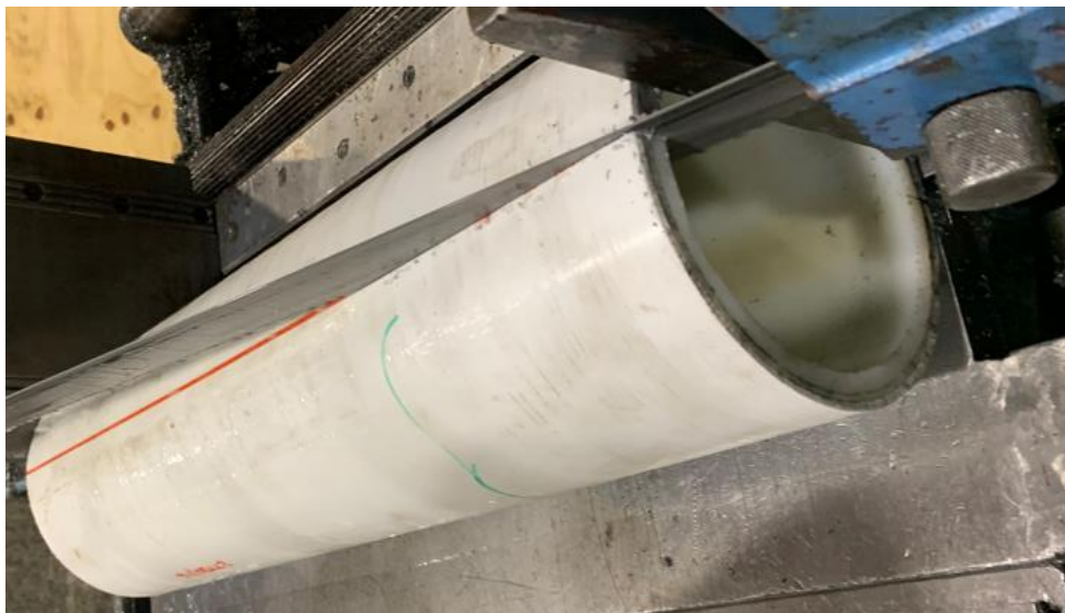
Figure 4-6 Pipe segments cut into halves
