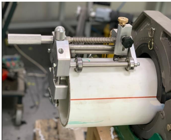
Figure 4-4 Rotary scraping for the pipe end
