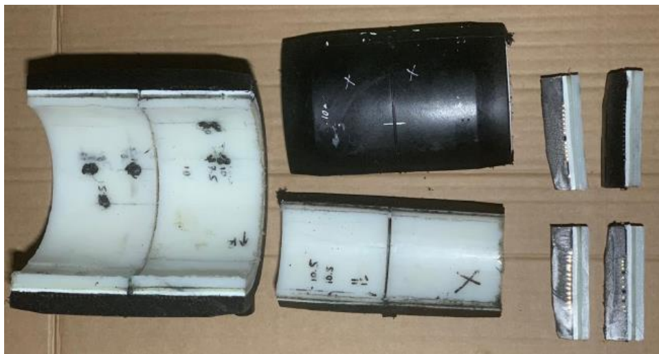
Figure 4-26 EF joint cut samples
