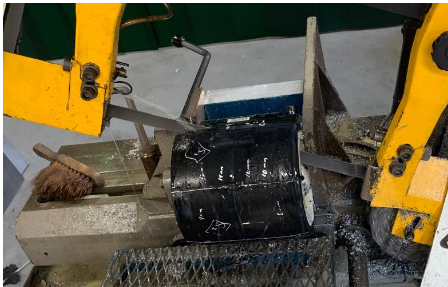
Figure 4-25 EF joint bandsaw cutting
