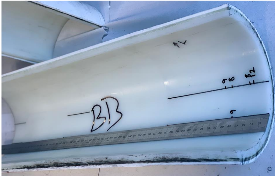
Figure 4-7 Marking thermocouple's location on the pipe
