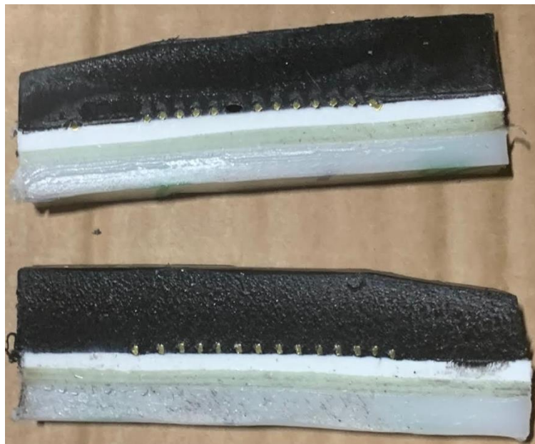
Figure 4-28 EF joint cut samples (contact wires) where potential full contact between pipe and fitting
