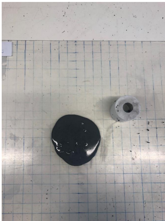
Figure 1. Picture of the example mini slump test after taking the measurements, with the white cone place beside (20mm grid).
