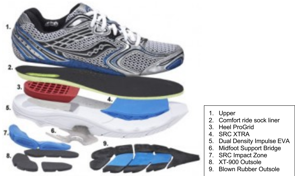
Figure 39: Saucony®'s ProGrid Jazz 12, schematic view of the running shoe construction (Saucony® Inc., 2017).
