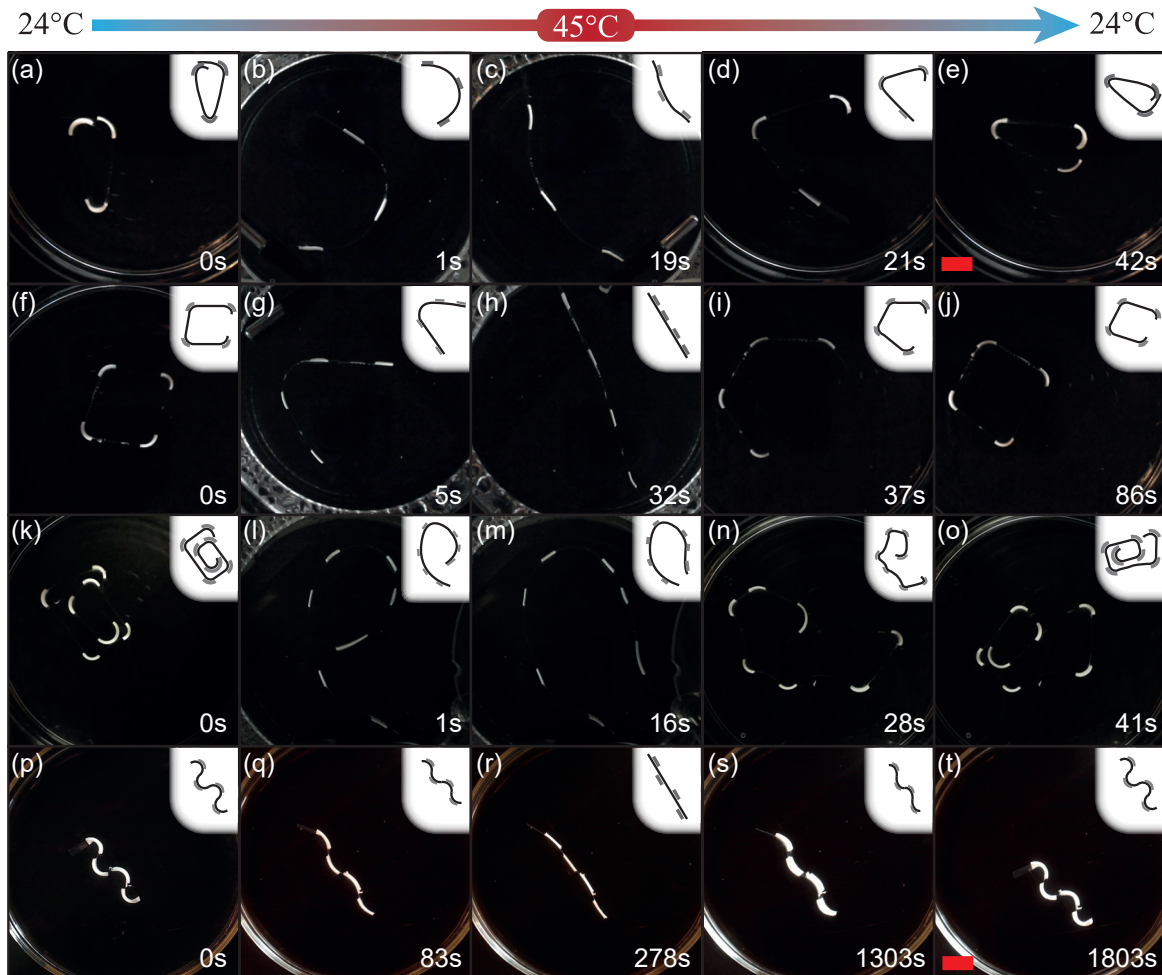
Fig. 4.8 Shape transformation of the pNIPAM/PVC soft strings: Triangle structure (a) self-unfolding into a string (b) and (c), and self-folding into a triangle (d) and (e). Square structure (f) self-unfolding into a string (g) and (h) and self-folding into a square (i) and (j). Shape transformation of the rectangular coil (k) into a string (l) and (m) and reversed transformation (n) and (o). Self-unfolding of the Acordeon string from (p) to (r) and self-folding from (r) to (t). For all pictures, scale bars are 10 mm
