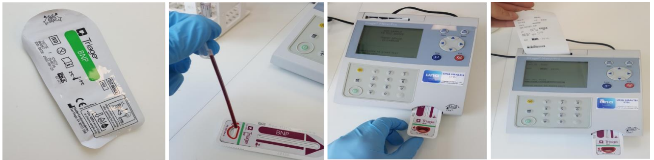
Test kit in foil packet Pipetting blood in the port Inserting sample Results printed
