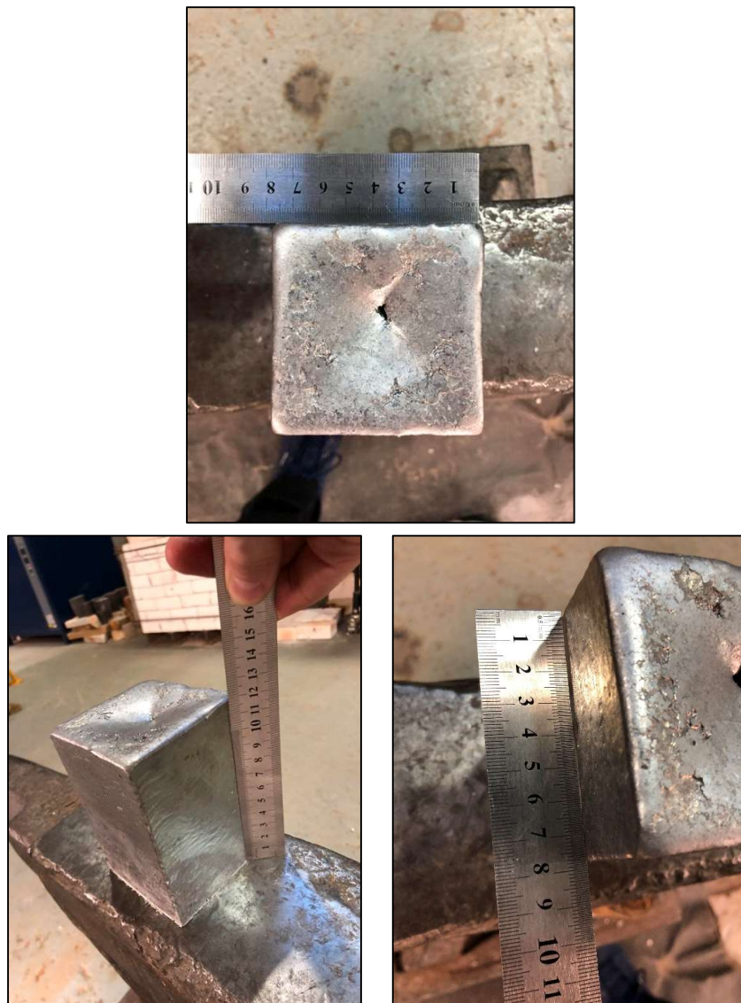
Figure 3.1: Images of the cast steel ingot, including the casting defect on the edge.
